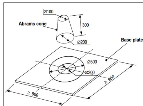
Figure 2 (a) Slump Flow
