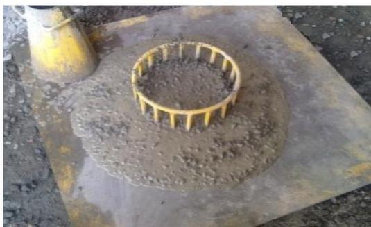
Figure 2 (b) Slump Flow
