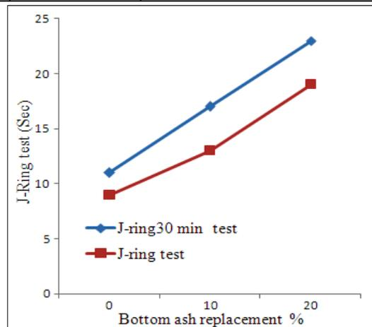
Figure 4 J-ring test results for different proportions of bottom ash
