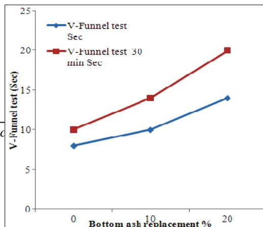
Figure 5 V-funnel test results for different proportions of bottom ash
