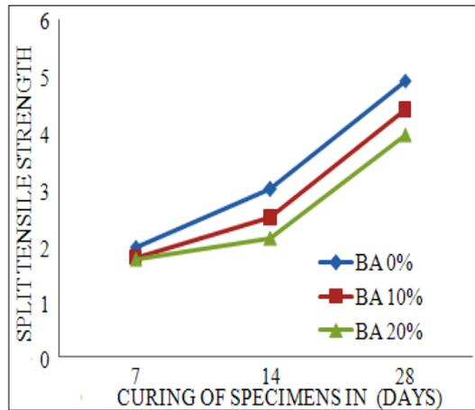
Figure 7 Split tensile strength of concrete with and without bottom ash
