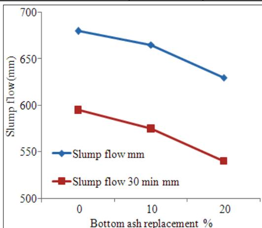
Figure 3 Slump flow of different proportions of bottom ash
