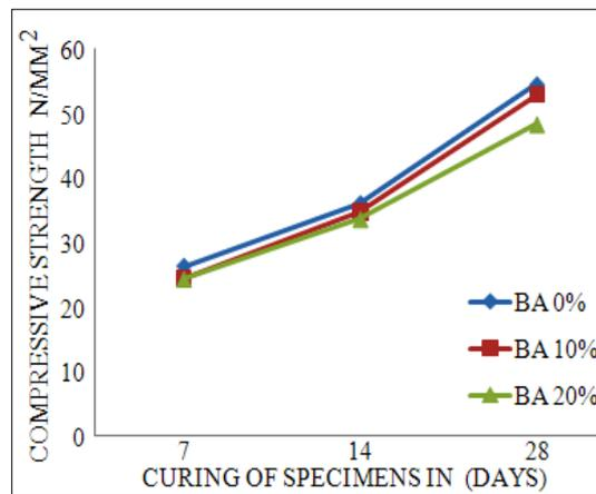
Figure 6 Compressive strength of concrete with and without bottom ash
