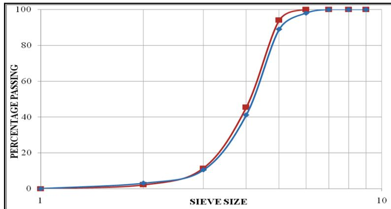
Figure 1 Particle size distribution curve for sand and bottom ash
