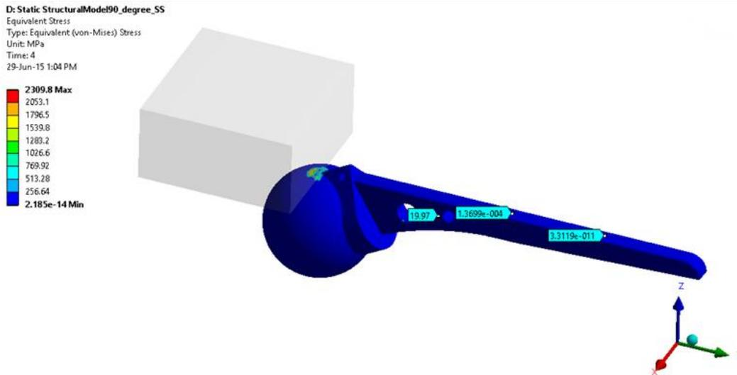
Figure 5(d): Von mises stresses at different strain gauge locations (3, 4, 6)
