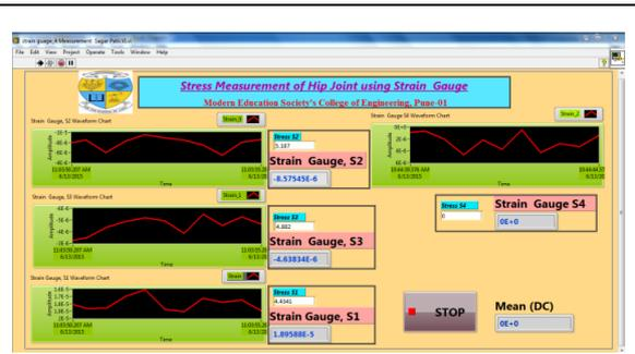
Figure 9: Value of the stress at 40<sup>0</sup> position
