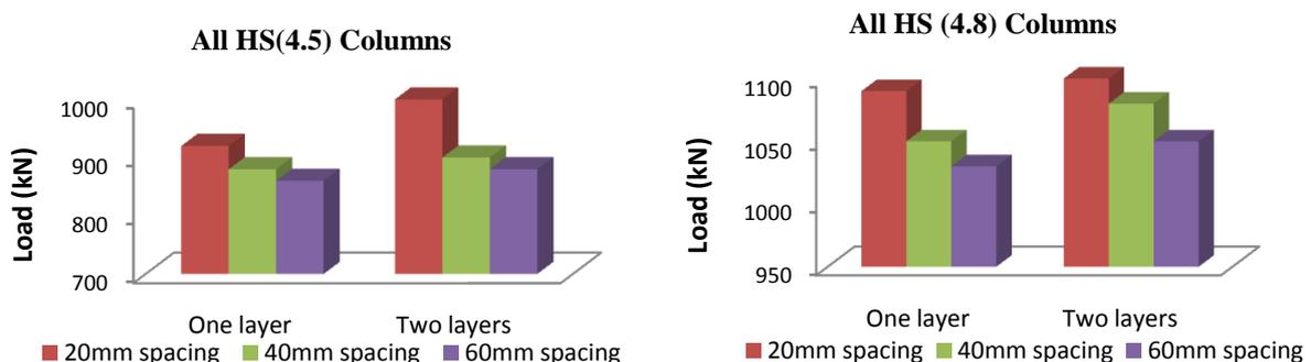
Fig.5 Ultimate load of all columns –Comparison
