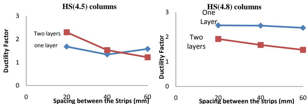
Fig. 7 Ductility Factor vs Spacing between the strips
