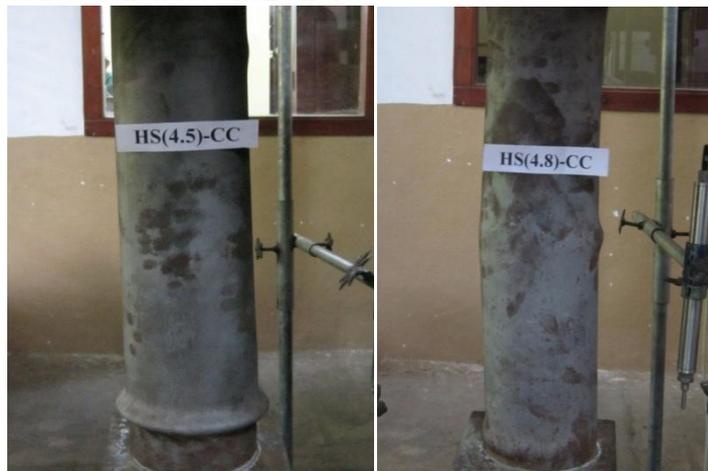
Fig. 2 Failure modes of Control Columns
