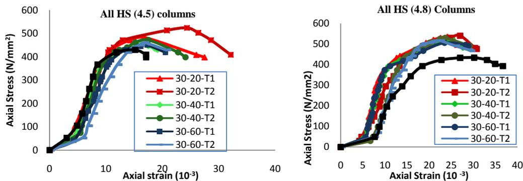
Fig.4 Axial stress -strain behaviour- comparison
