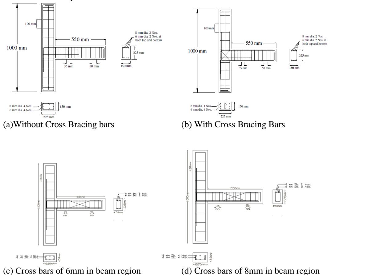
Figure 1. Reinforcement details of specimen of (a) Without Cross Bracing bars and (b) With Cross Bracing Bars. (c) Cross bars of 6mm in beam region. (d) Cross bars of 8mm instead of 6mm in beam region.
