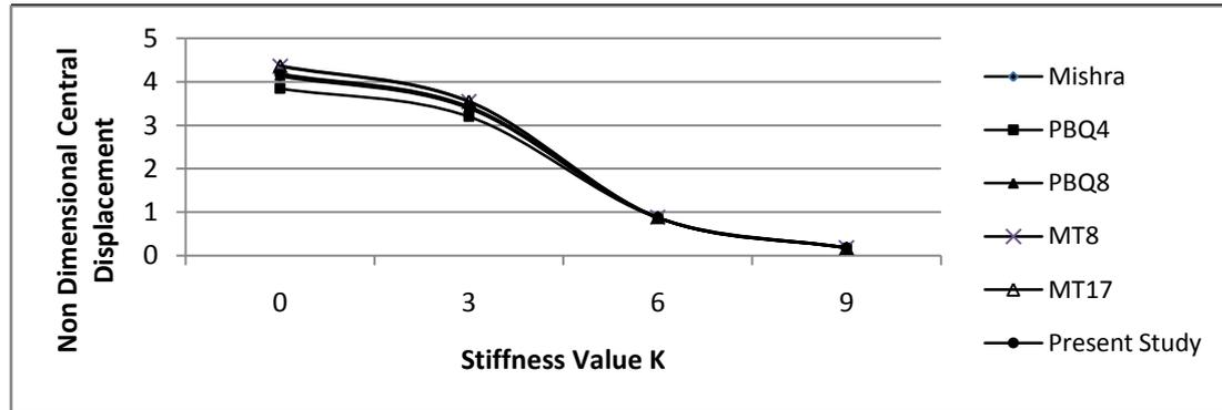
Figure 4. Non-dimensional central displacement of simply supported plates with different K values subjected to uniformly distributed load
