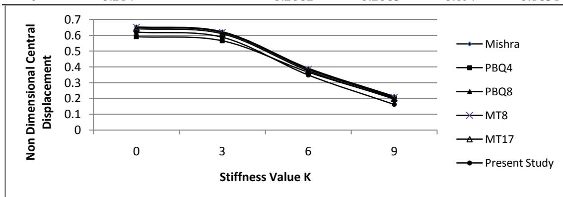
Figure 3. Non-dimensional central displacement of clamped plates with different K values subjected to concentrated load
