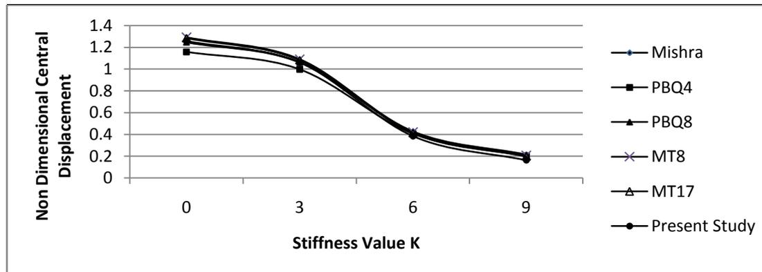
Figure 5. Non-dimensional central displacement of simply supported plates with different K values subjected to concentrated load
