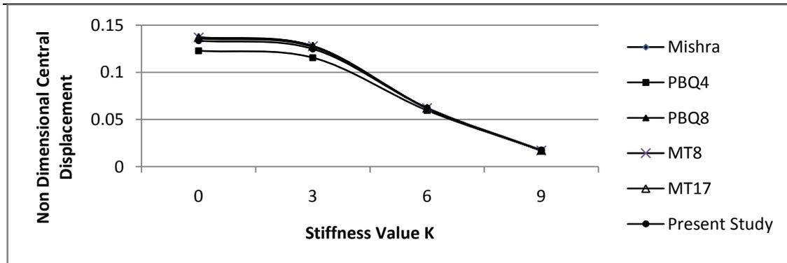
**Figure 2. Non-dimensional central displacement of clamped plates with different K values subjected to udl**
