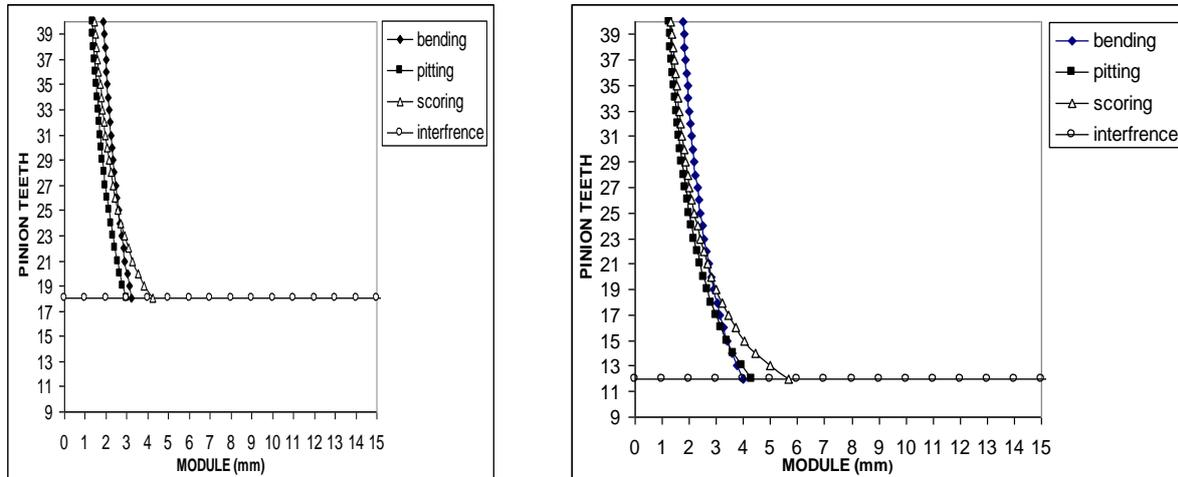
**Figure 4.3 and 4.4 : Feasible design space, Torque=100.5(N-m), n1=1120, m<sub>G</sub> =2,  $\Phi= 20^\circ$  and  $\Phi= 25^\circ$**
