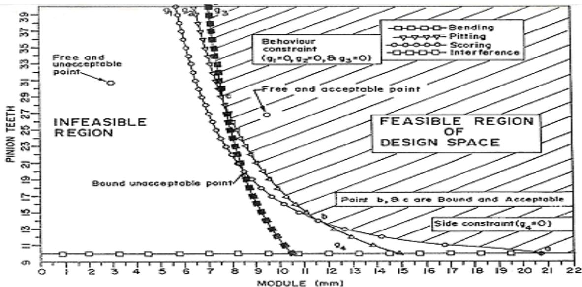
**Figure3.3: Design space for compact spur gear**
