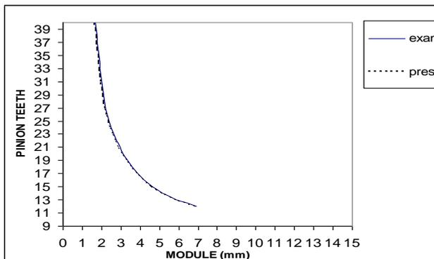
Figure 4.2 Comparison between  $m_{max}$  curves, Torque=600.5(N-m),  $n_1=1000$ ,  $m_G=1.5$
