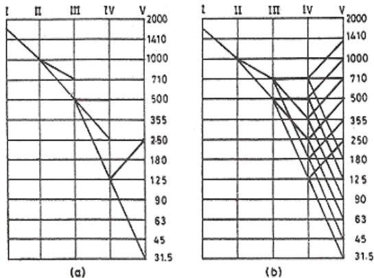
Figure 4.1: (a) Ray diagram (b) Speed chart
