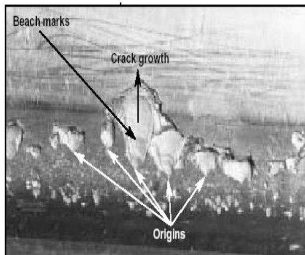
**Figure.3.1: Bending fatigue fracture of gear teeth**      **Figure.3.2: Surface fatigue fracture of gear teeth**
