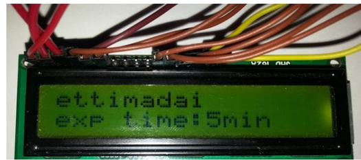
Fig. 4 LCD display showing the current position of the bus and expected time
