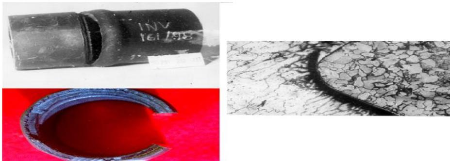
Fig: 3 Tube failures because of dissimilar welds.
