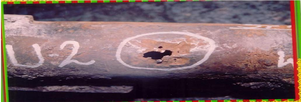
Fig:5 Tube failures due to caustic corrosion.
