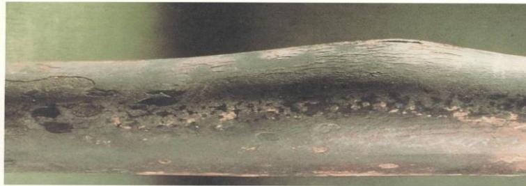
Fig: 2 Tube failed due to high temperature creep.
