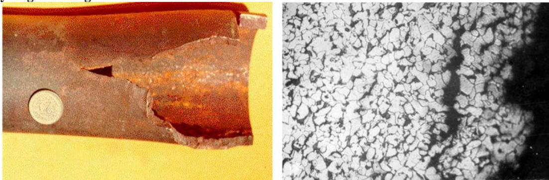
Fig: 6 Tube failures because of hydrogen damage.
