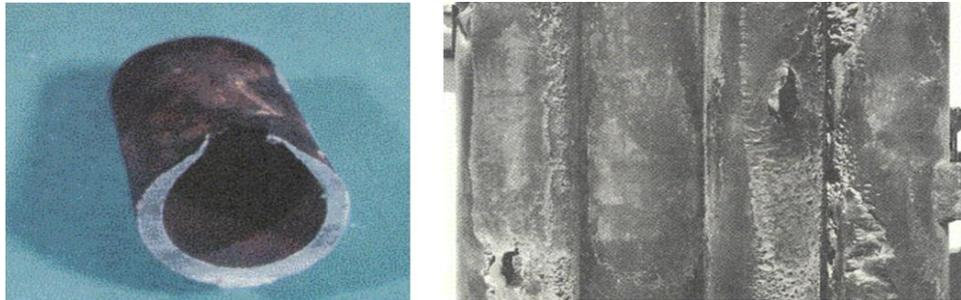
Fig: 9 Tube failures due to fly ash erosion
