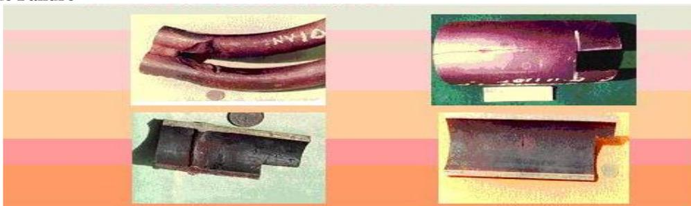
Fig: 7 Tube failures because of fatigue failure.
