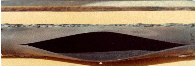
Fig: 1 Tube failed due to short term overheating
