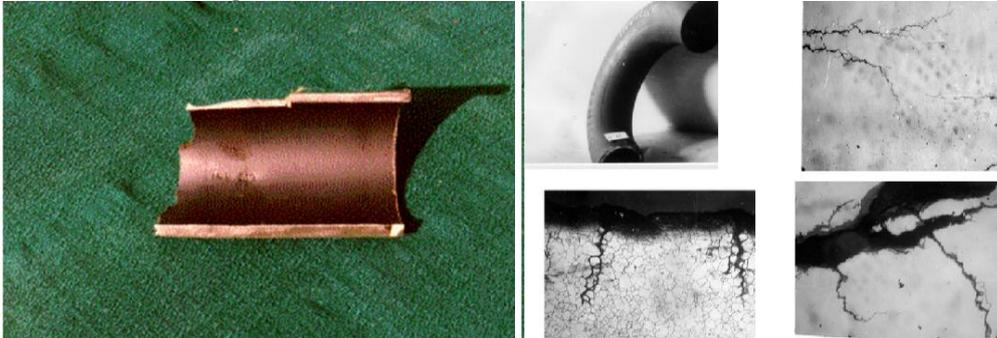
Fig: 8 Tube failure due to stress corrosion cracking.
