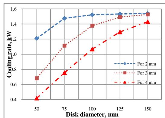
Fig. 5: Cooling rate per unit length of device for various diameters and pitch of disk
