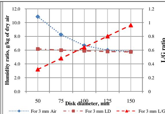
Fig. 7: Variation of humidity ratio for various disk diameters and L/G (liquid to gas flow) ratio
