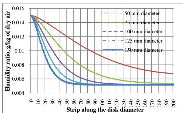
Fig. 4: Variation of humidity ratio of air along the diameter of the disk (depth of the channel)
