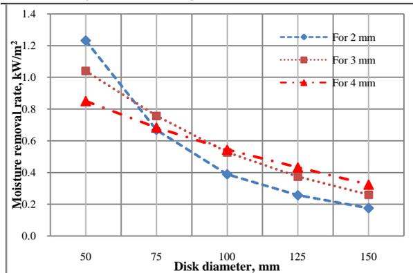
Fig. 6: Cooling rate provided by RDCD per unit length at various disk diameter and pitch
