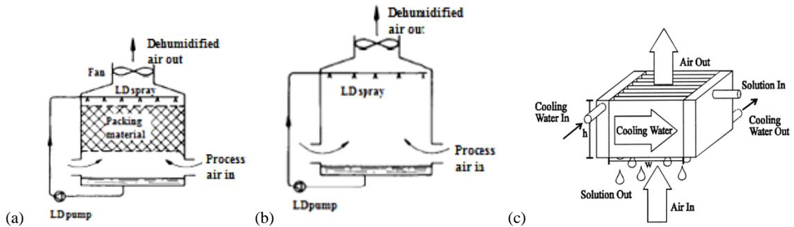
Fig. 1: Various types of LD-air contacting devices (a) Packed bed (b) Spray tower (c) Falling film
