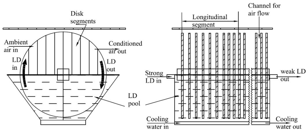
Fig. 3: Configuration and methodology of simulation for RDCD
