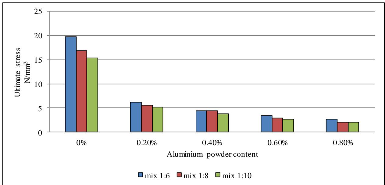
Fig 4.1 Strength Comparison of Specimens for 7-Days (Quarry Dust)
