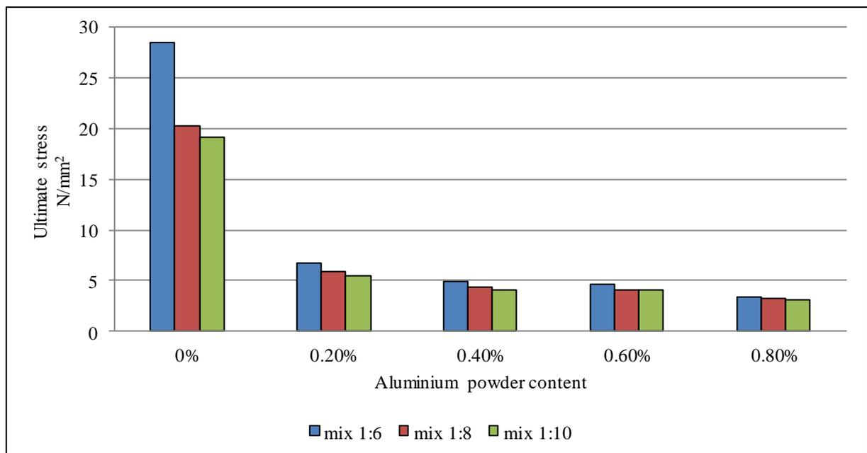
Fig 4.2 Strength Comparison of Specimens for 28-Days (Quarry Dust)
