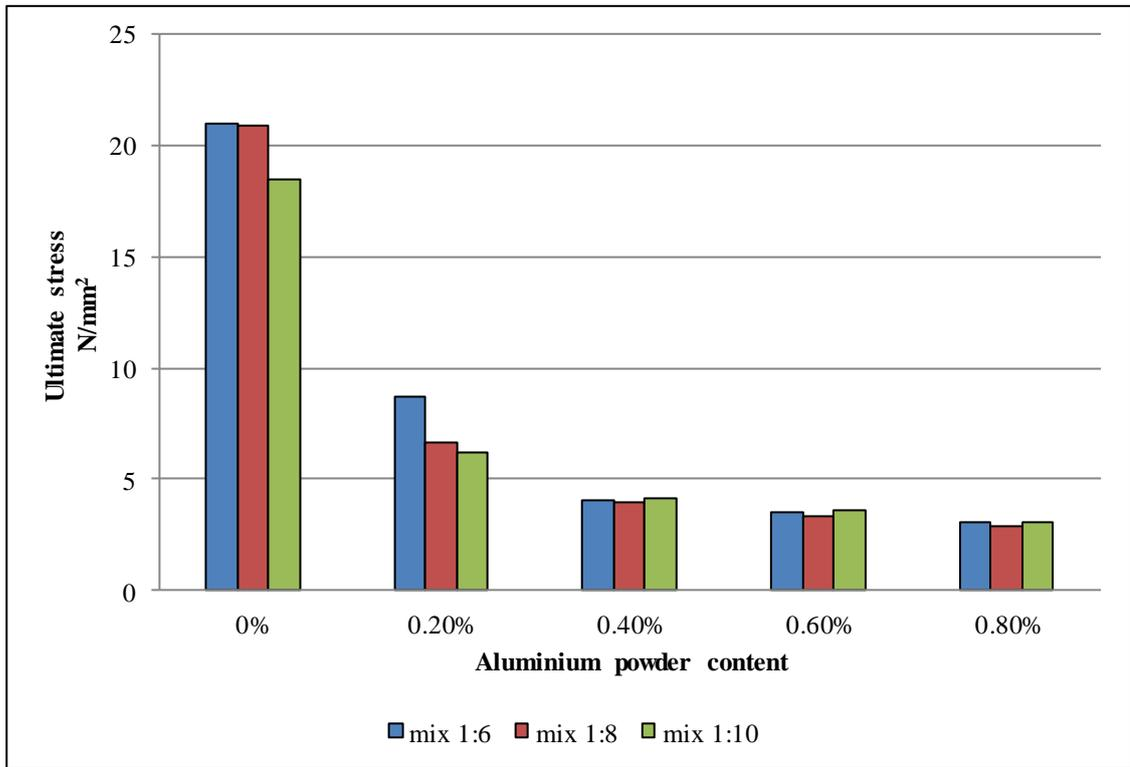
Fig 4.3 Strength Comparison of Specimens for 7-Days (Sand)
