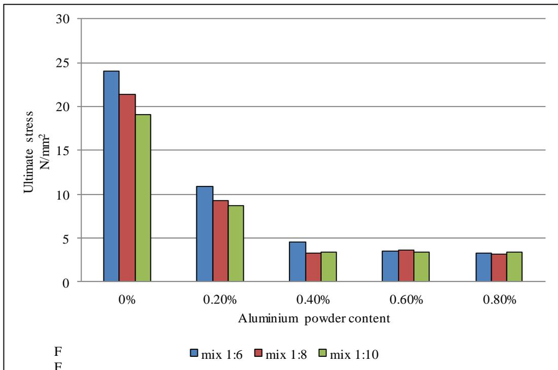
Fig 4.4 Strength Comparison of Specimens for 28-Days (Sand)
