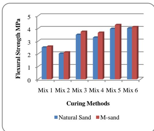
Fig. 5 Flexural strength for 7 days
