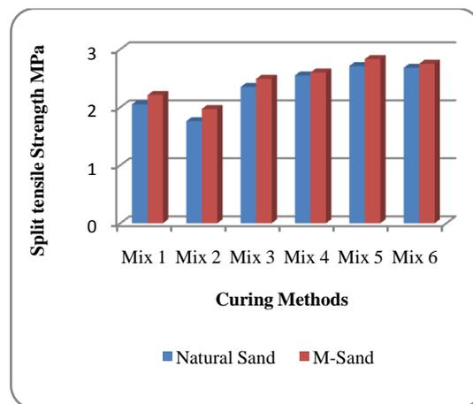
Fig. 4 Split tensile strength for 28 days
