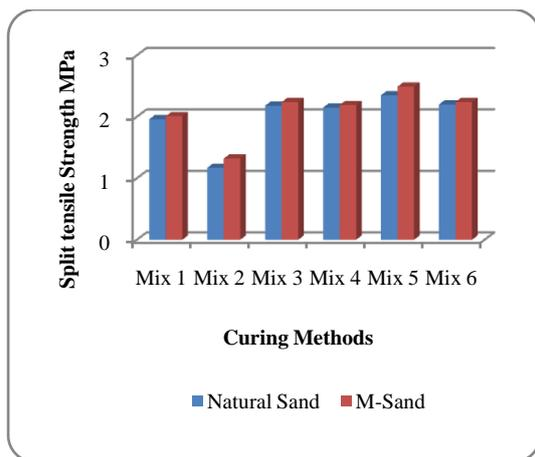
Fig. 3 Split tensile strength for 7 days
