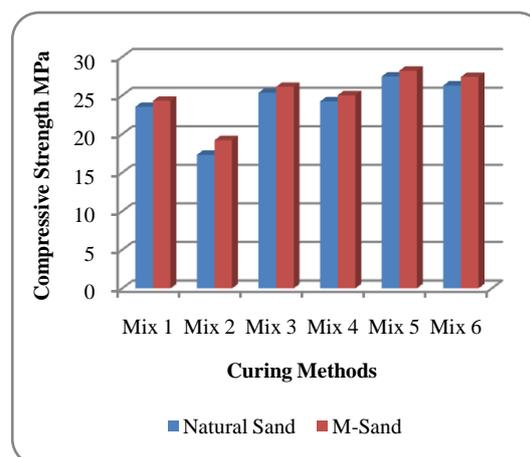
Fig. 2 Compressive strength for 28 days
