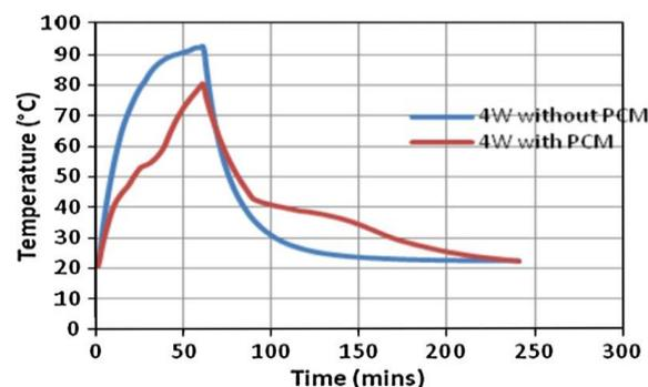
Fig. 5. Overall (average) performance of the heat sinks
