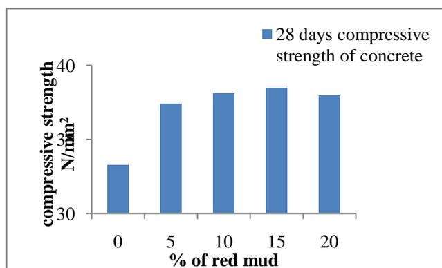
Figure 1. 28 Days Compressive strength of red mud concrete without hydrated lime
