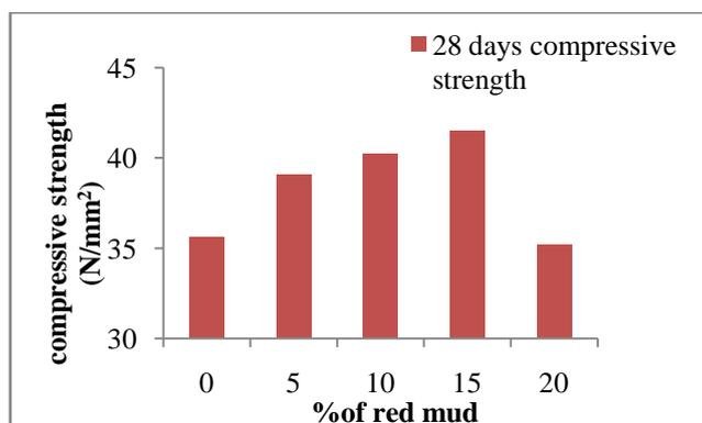
Figure 2. 28 Days Compressive strength of red mud concrete with hydrated lime
