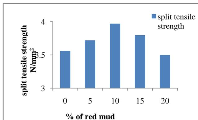
Figure 3. 28 Days split tensile strength without hydrated lime
