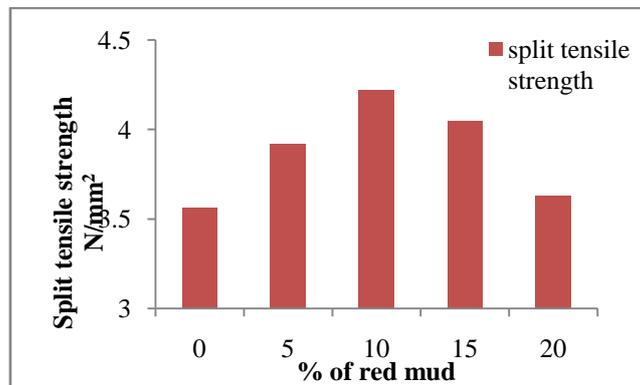
Figure 4. 28 Days Split tensile strength with hydrated lime
