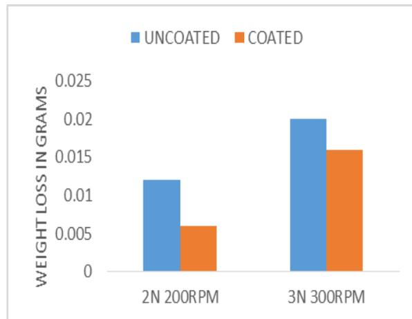
Figure 3.8 comparison of weight loss due to wear for the coated and the uncoated specimen
