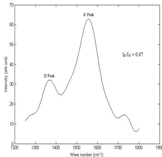
**Figure 3.4 Raman Spectroscopy of the DLC coated film**
