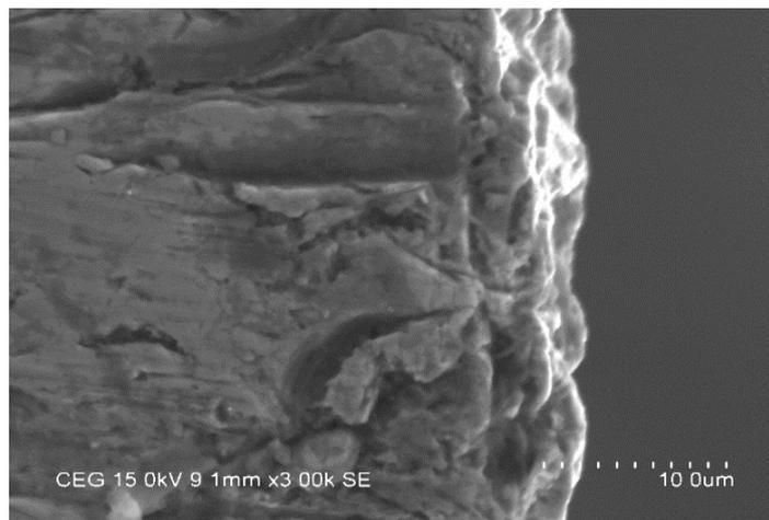
**Figure 3.2 Adhesiveness of the DLC film with the substrate**
