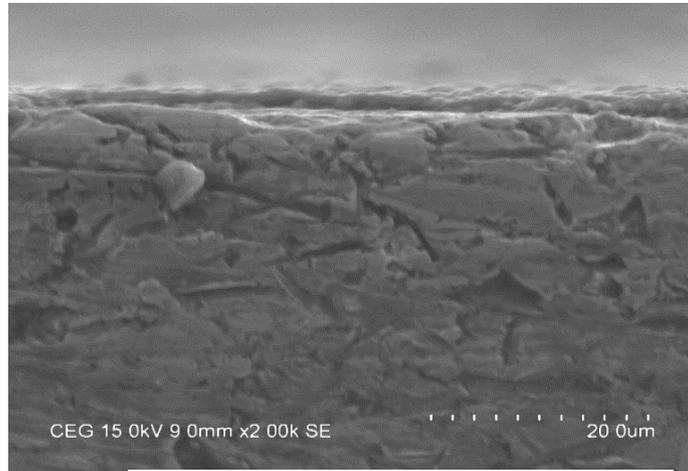
**Figure 3.1 Thickness of the coated film**
