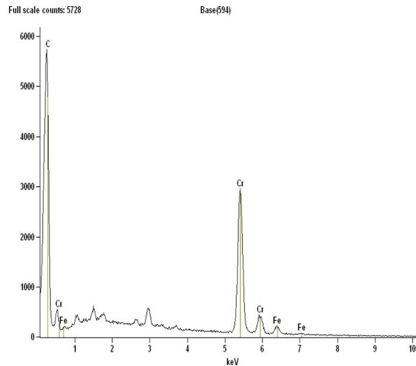
**Figure 3.3 EDX analysis of the DLC film**
