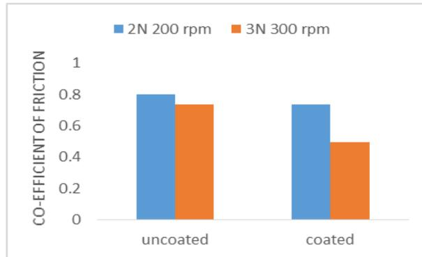
Figure 3.5 coefficient of friction Vs Coated/Uncoated material
