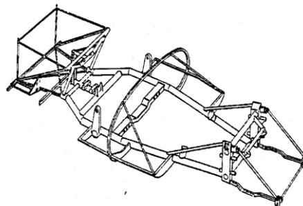
Figure 2.2: Twin-tube chassis
