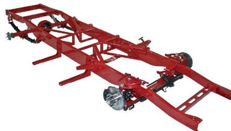
Figure 1.5: Sample of the Truck Chassis
