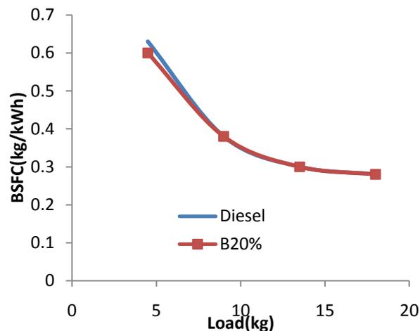
Fig :2 Load vs Brake Specific Fuel Consumption
