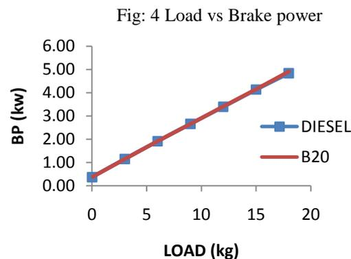
Brake power is the power output of the drive shaft of an engine without the power loss caused by gears, transmission, friction, etc. It's called also pure power, useful power, true power or wheel power as well as other terms.
