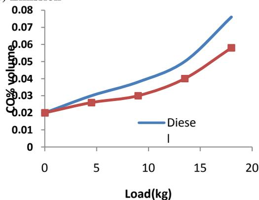
**Fig:4 Load vs Carbon Monoxide Emission**
