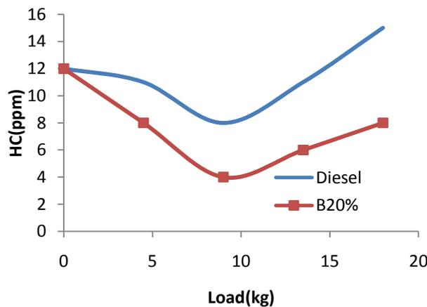
**Fig :5 Load vs Hydrocarbon Emission**
