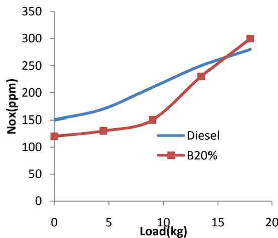
**Fig : 6 Load vs NOx Emission**
