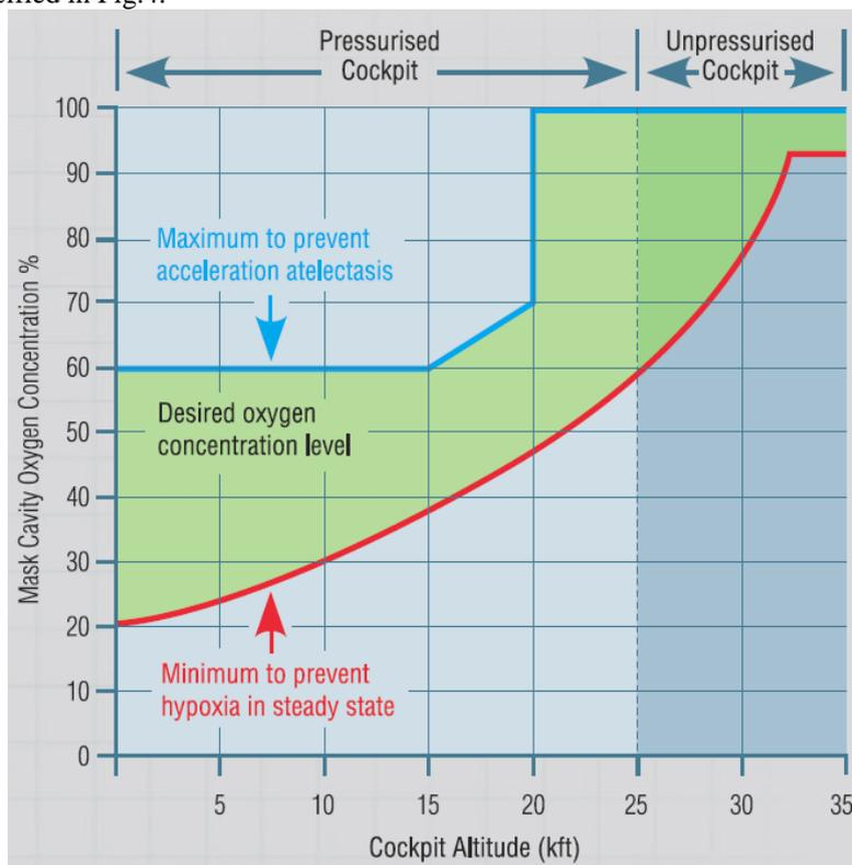
Fig.4. Variation of oxygen concentration with altitudes
