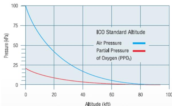
Fig.1. Variation of air pressure & PPO<sub>2</sub> with altitudes
