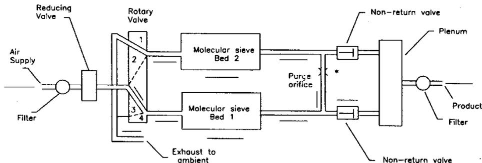
Fig.3 Typical two bed molecular sieve system
