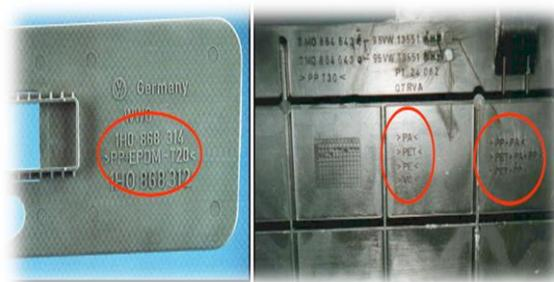
**Fig.6. Material marking**
