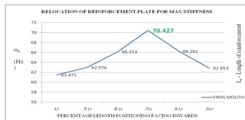
**Figure: 8.1 Relocation of reinforcement plate for max stiffness**
