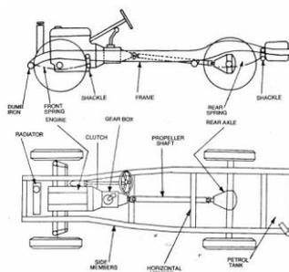
**Figure 2.1: chassis frame**
