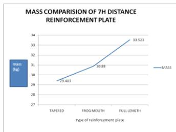
Figure: 7.1 Mass comparison of 7H distance reinforcement plate
