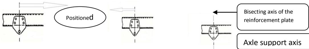
**Figure: 5.1** Aligned towards the centre of the chassis frame from the support axis **Figure: 5.2** Aligned away from the centre of the chassis frame from the support axis **Figure: 5.3** Aligned on the support axis with the middle axis **Figure: 5.4** Aligned on the support axis with the middle axis
