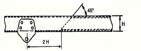
Figure: 4.3 Tapered reinforcement
