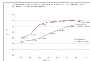
Figure: 7.2 Comparison of natural frequency shift with tapered and frog mouth reinforcement
