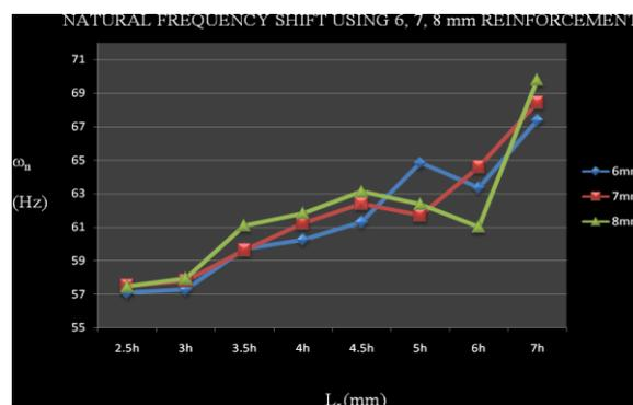
**Figure: 6.1** Natural frequency shift using 6, 7, 8 mm reinforcement plates
