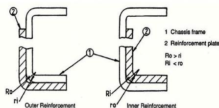
Figure: 4.1 Chassis reinforcement
