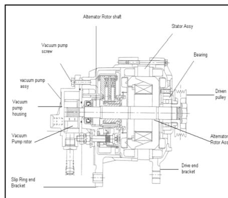
Fig 1.1 Alternator Section View
