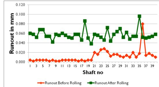
**Fig 3.4 Spline Runout Shift wise –Multi Vari Chart**
