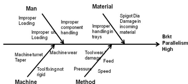
**Fig 3.1 Cause and Effect diagram – bracket Machining**
