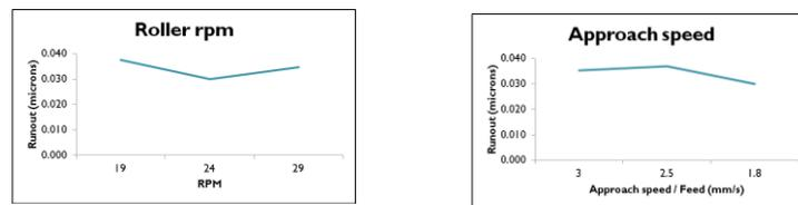
**Fig 3.7 Mean Analysis – RPM and Approach Speed**
