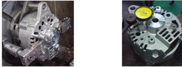
Fig 3.2 Bracket Machining and Parallelism Measurement
