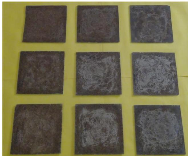
Fig 1- Photographic image of fabricated Composite sheets
