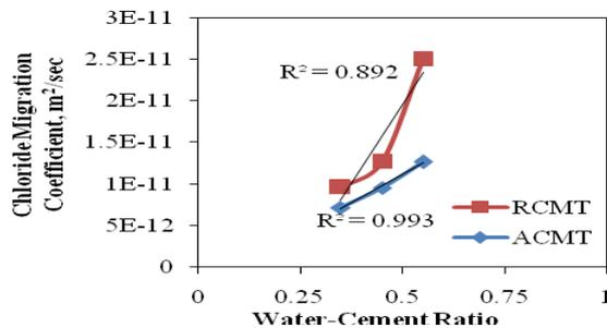
Fig. 4 Graph between Water- cement ratio and Chloride migration coefficient.
