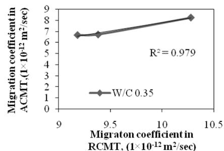
Fig 5c Correlation between migration coefficient in RCMT and ACMT for water-cement ratio 0.35
