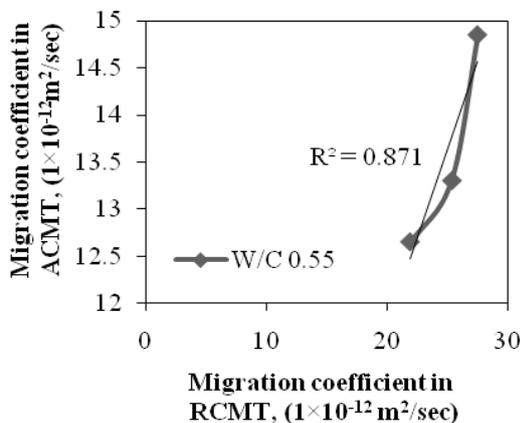
Fig 5a Correlation between migration coefficient in RCMT and ACMT for water-cement ratio 0.55
