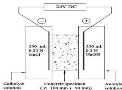
Fig 3 Arrangement of ACMT setup
