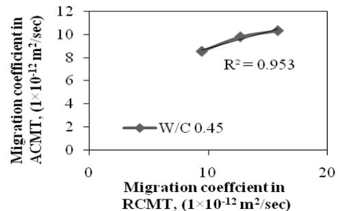
Fig 5b Correlation between migration coefficient in RCMT and ACMT for water-cement ratio 0.45
