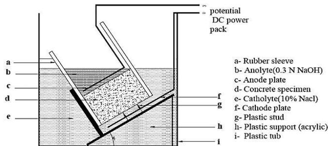
Fig 1 Arrangement of RCMT setup
