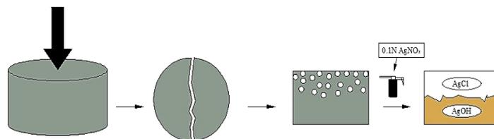
Fig 2 Schematic representation of colourimetric method
