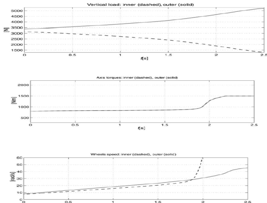
Fig.3 Graphical representation of the vertical loads, axial torques, and rotation speed of the inner & outer wheel
