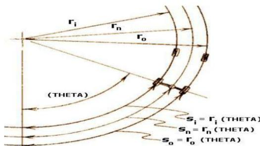
Fig.1 Turning radius diagram
