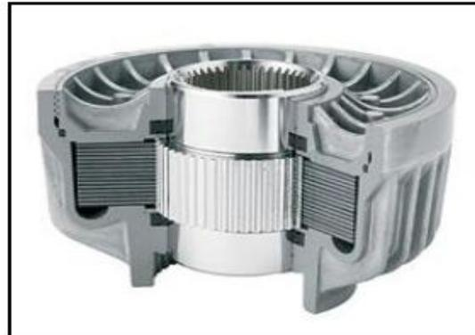
Fig.5 Viscous limited slip differential
