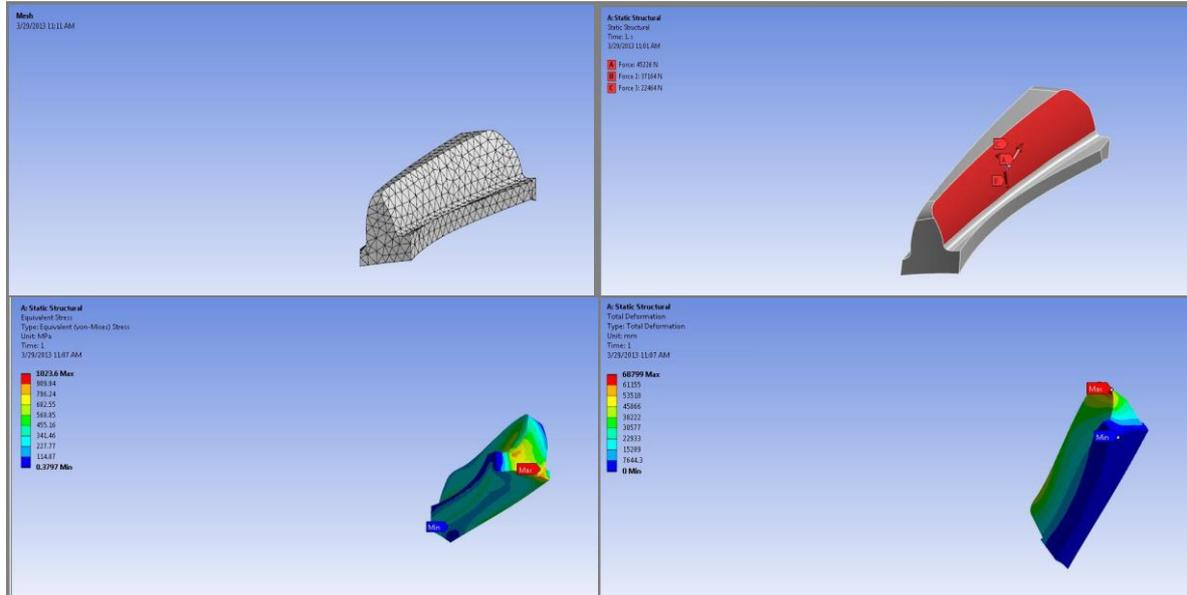
Fig.9 Finite element analysis of crown gear tooth
