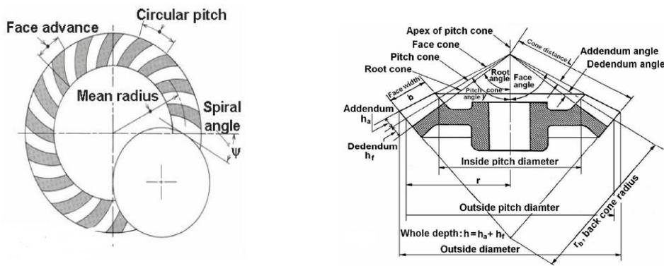
Fig.7 Bevel gear terminology
