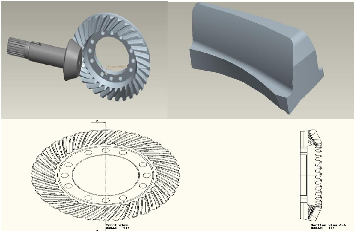
Fig. 8 3-D model of assembly and tooth 2-D view of Crown gear
