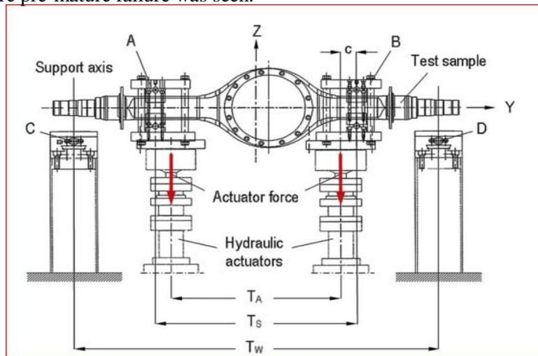
Fig.-10. Schematic for fatigue test [2]
