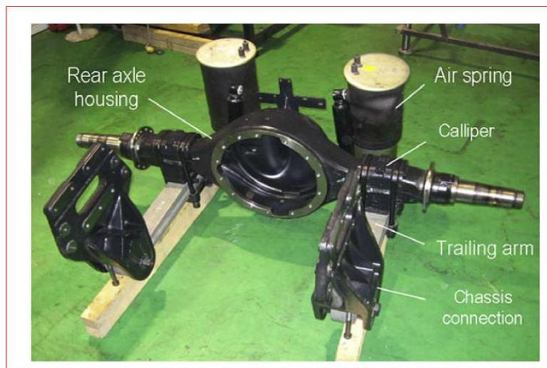
Fig.-8. Rear axle assembly of a commercial vehicle [2]
