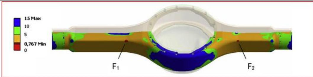
Fig.-13. Factor of safety distribution on lower shell [2]
