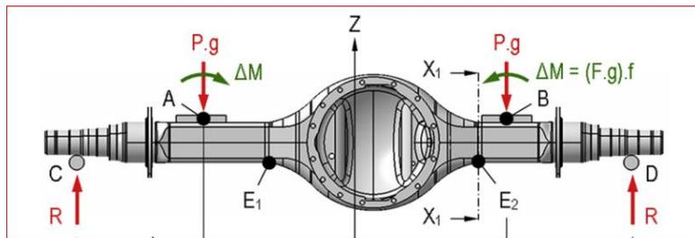
Fig.-9. Applied loads on a housing [2]
