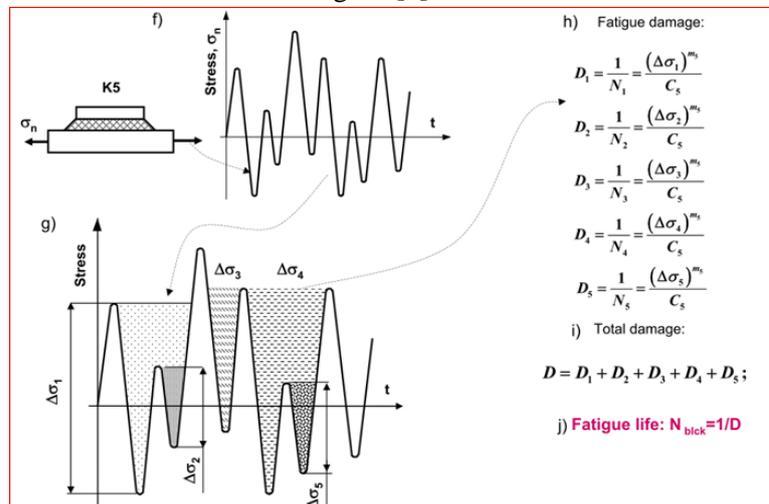
Fig.-3.(Steps in fatigue life prediction by stress approach) [1]
