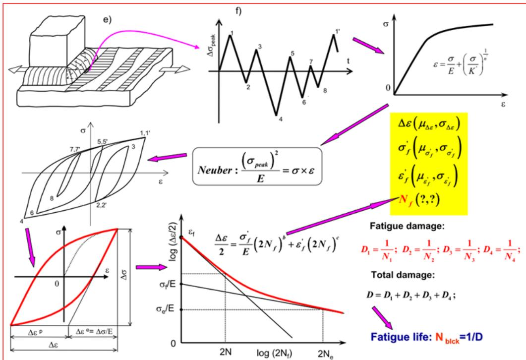
Fig.-5. (Steps in fatigue life prediction by strain approach) [1]
