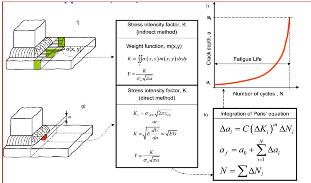
Fig.-7. (Steps in fatigue life prediction by fracture mechanics approach) [1]
