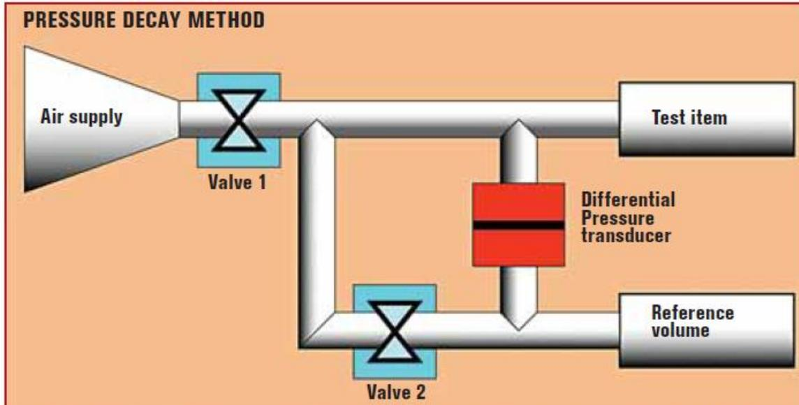
Test item and reference volume are pressurized and then isolated from the source by closing valve 1. Reference volume is then isolated from test item by closing valve 2, but they remain connected by a differential pressure transducer. Transducer reads pressure differential between non-leaking reference volume and leaking test item twice over a known time interval. The leak rate is calculated from the change in pressure, and the time over which it occurred.
