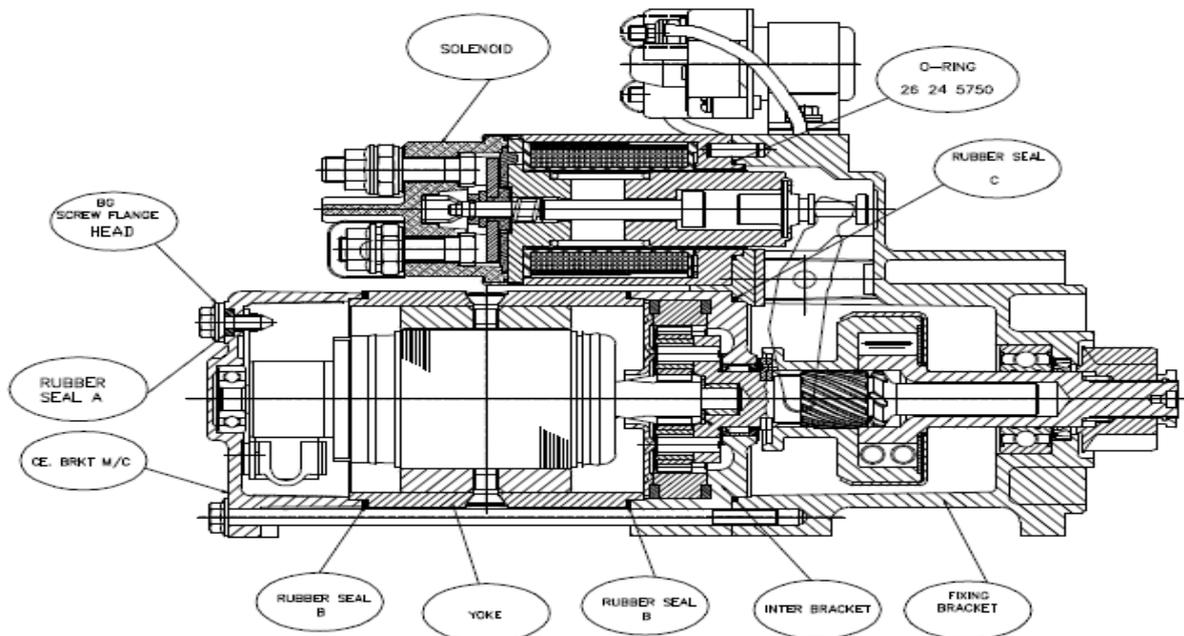
Fig. 1.1 Gear Reduction Starter Sectional view
