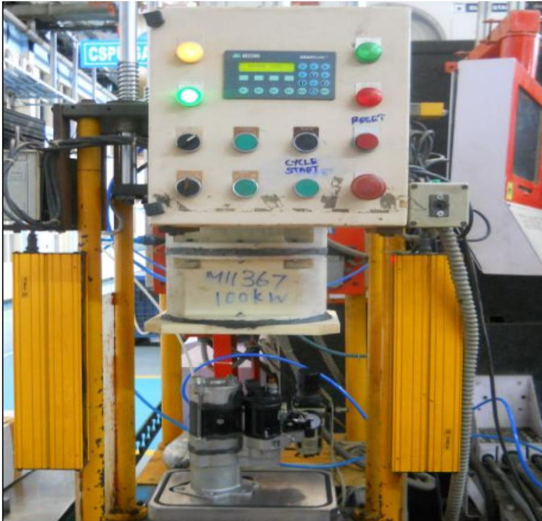
**Fig 3.3 Photograph of Air leak test rig**
