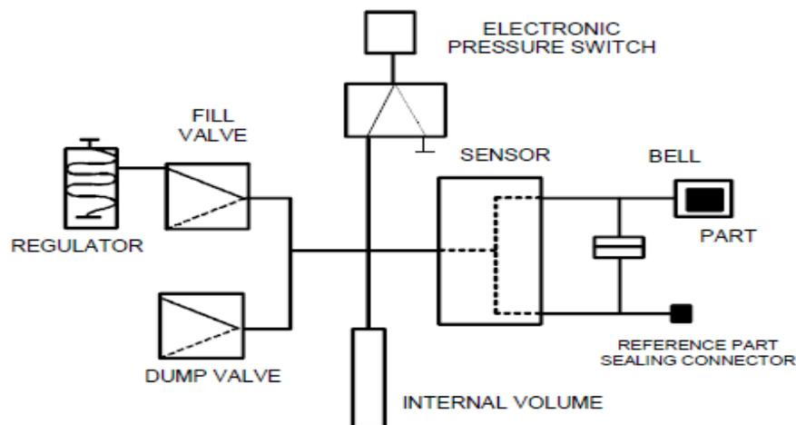
**Fig 3.2 Sealed component measurement**
