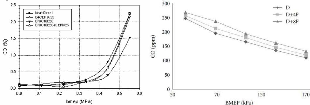
Figure-4 Variation of CO with BMEP with respect to engine load at 2200 rpm
