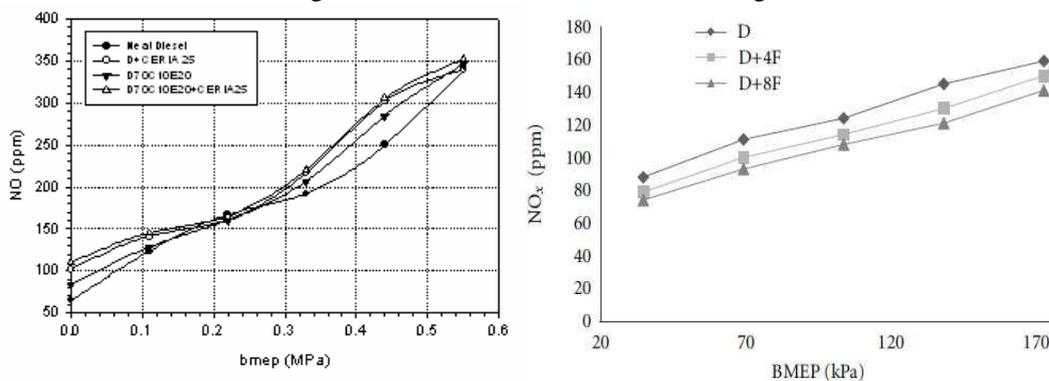
Figure-5 Variation of NO<sub>x</sub> with BMEP with respect to engine load at 2200 rpm
