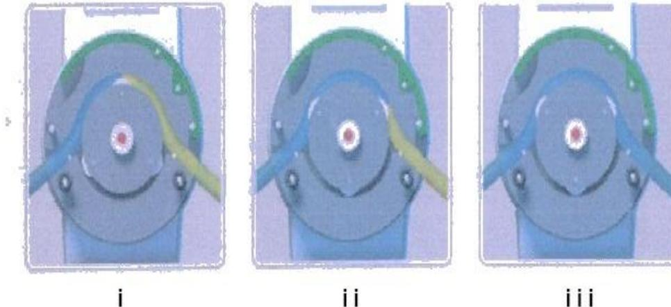
Figure 3.2.1: Principle of peristaltic pump
