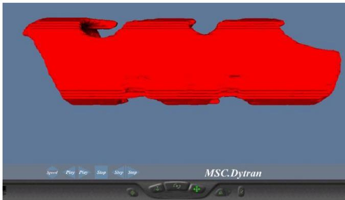
Fig.5.17 Iteration 4: Sloshing of LPG in a tank with two modified baffle showing peak amplitude of fluid
