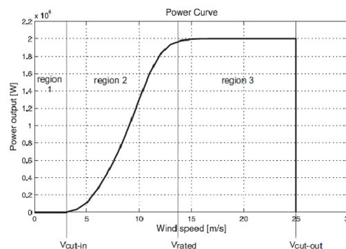
Fig1. Power o/p Vs Wind speed
