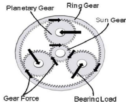
Fig 4b.-Planetary Gear Set Loads
