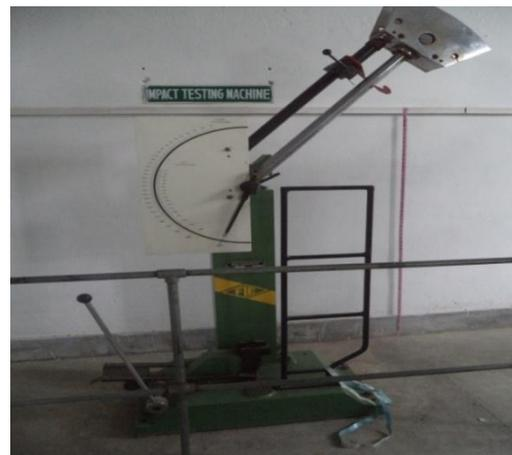
**Fig: 3 Charpy Impact Testing machine**
