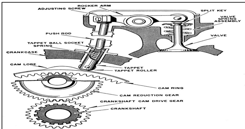
Fig.1 Valve Train Mechanism
