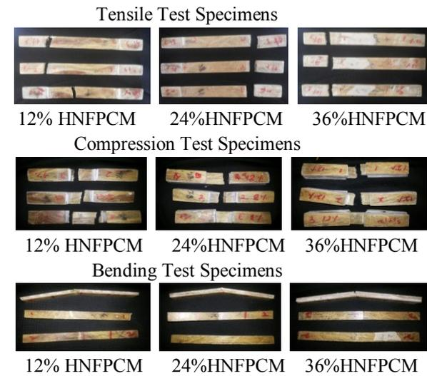
Fig 3.1: Fabricated Specimens Before and After Testing
