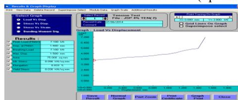
**Table 4.1:** Tabular column shows Experimental results (Graph) of Tensile Test 12% HNFPCM.
