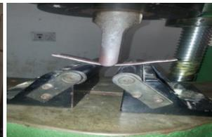
Fig 3.5: Bending Testing
