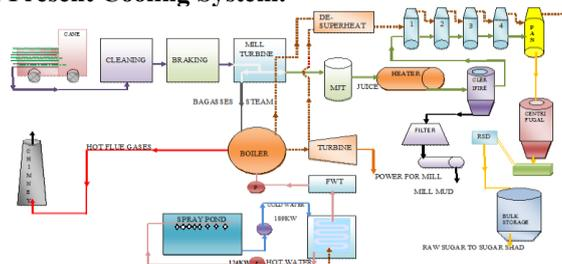
Fig.1.1 Raw Sugar Milling with Present Cooling System
