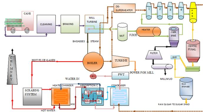
Fig.1.2 Raw Sugar Milling with Proposed Cooling System
