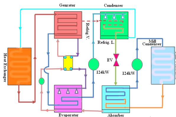
Fig. 1.3 Absorption Chiller with Proposed Cooling System
