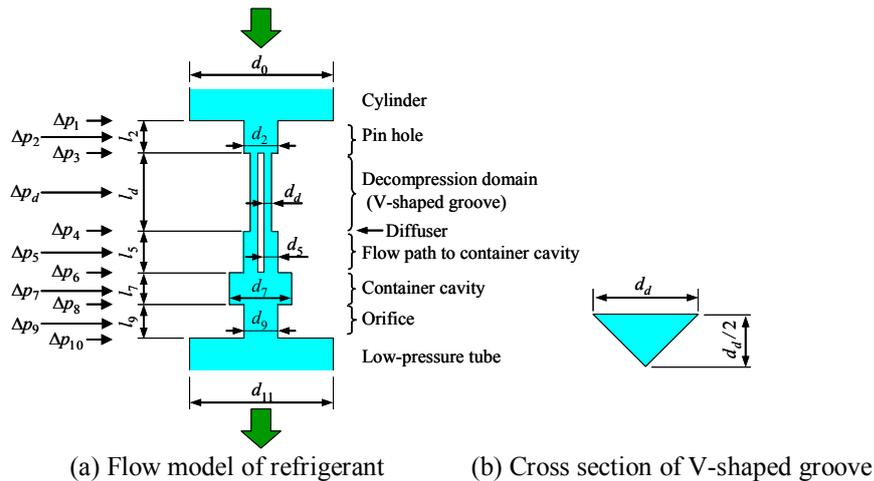
**Figure 4** Flow model for pulse driven-type electromagnetic control expansion valve
