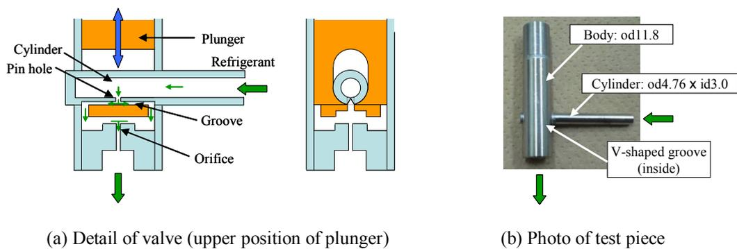
Figure 2 Pulse driven-type electromagnetic control expansion valve
