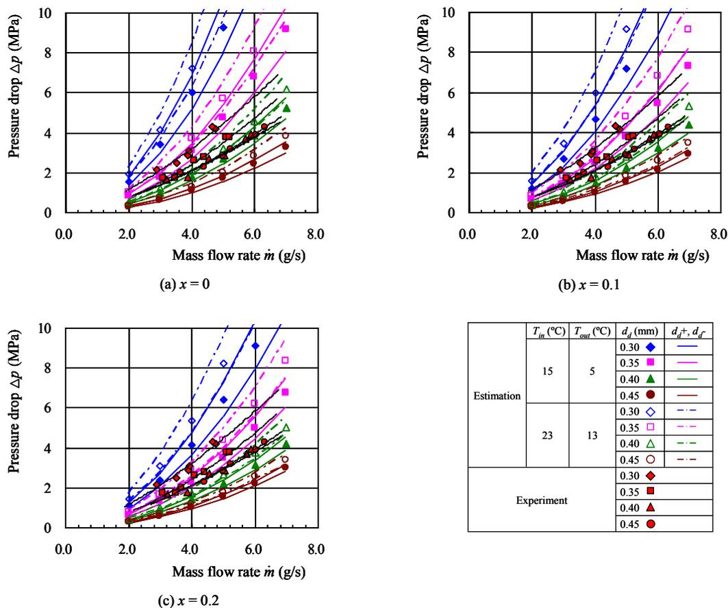
Figure 5 Experimentally obtained pressure drop and theoretical estimation
