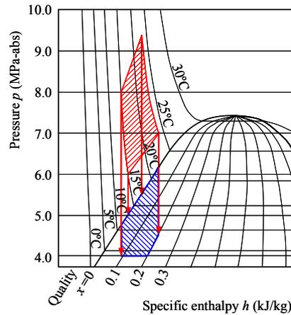
**Figure 3** A part of the R744 Mollier chart for the experimental conditions
