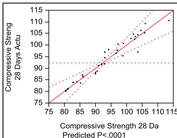
**Figure( 6) The Actual 28 days Compressive strength (MPa) and the Predicted 28 days Compressive strength (MPa) (as per JMP Modeling)**
