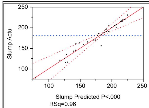
Figure (7) The Actual Slump (mm) and the Predicted Slump (mm) (as per JMP Modeling)
