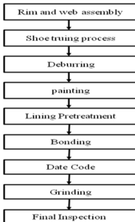
Figure 2. Process Flow
