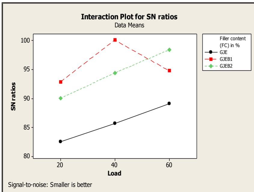
Figure 4: Interaction graph between normal load and filler content for specific wear rate
