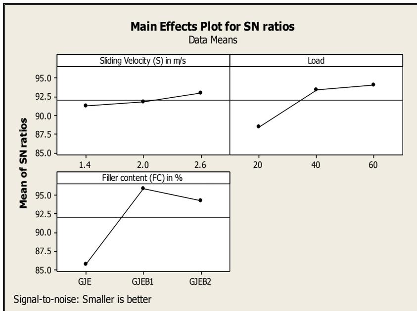
**Figure 1:** Effect of control factors on specific wear rate of hybrid composites
