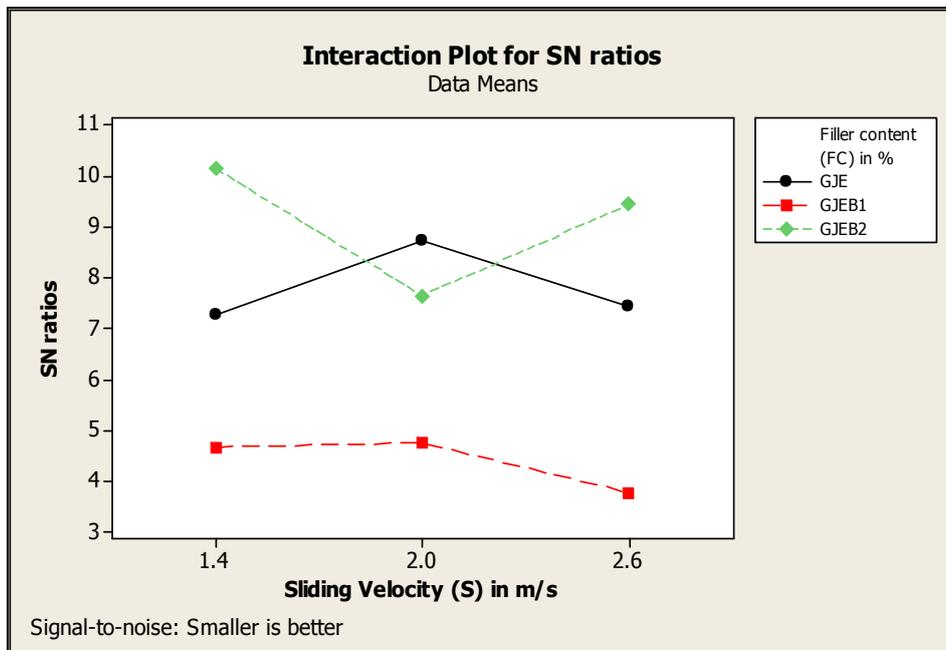
**Figure 7:** Interaction graph between sliding velocity and filler content for coefficient of friction
