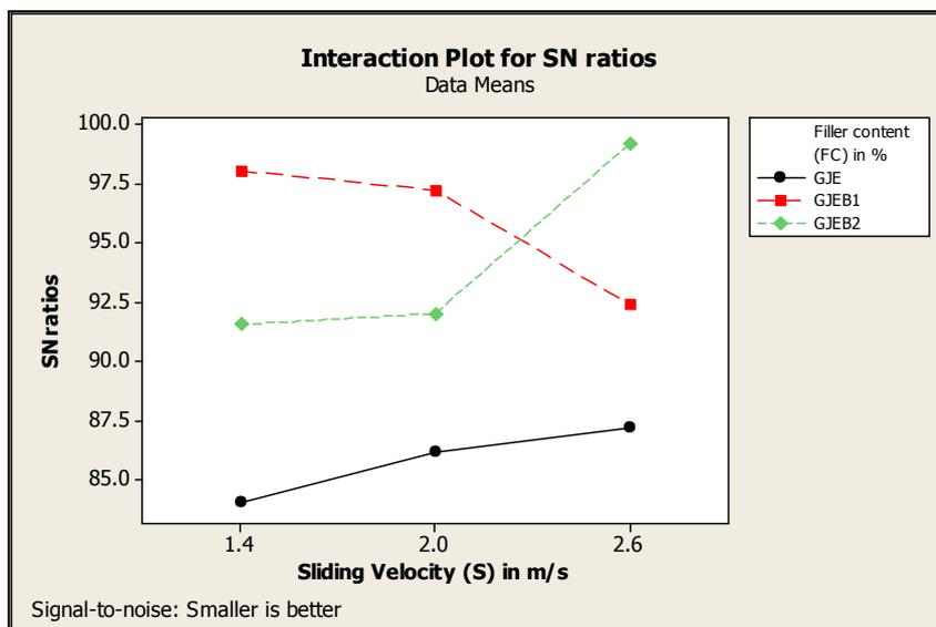
**Figure 2:** Interaction graph between sliding velocity and filler content for specific wear rate
