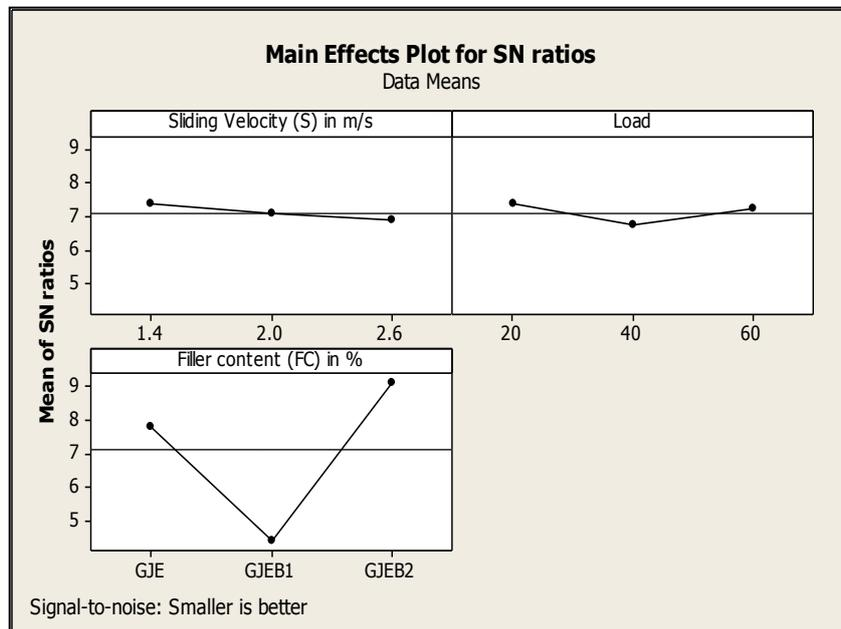
**Figure 5:** Effect of control factors on COF hybrid composites
