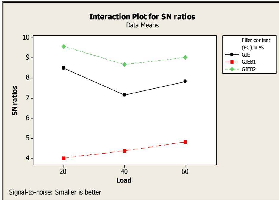
Figure 8: Interaction graph between normal load and filler content for coefficient of friction
