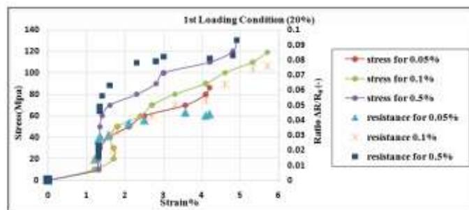
Fig 1: Graph Represents Curve Between Tensile Stress And Electric Resistance Corresponding To Stress of GFRP Modified With MWCNT-CNF For 1<sup>st</sup> Incremental Loading.
