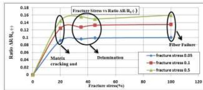
Fig 9: Relation of Loading Condition with Residual Resistance of MWCNT-CNF Epoxy Resin
