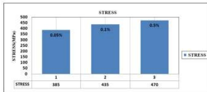
Fig 5: Typical Bar Graph Represents Tensile Stress Increasing Value of GFRP Modified With MECNT-CNF
