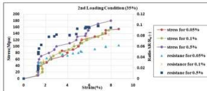
Fig 2: Graph Represents Curve Between Tensile Stress And Electric Resistance Corresponding To Stress of GFRP Modified With MWCNT-CNF For 2<sup>nd</sup> Incremental Loading.
