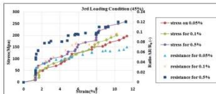
Fig 3: Graph Represents Curve Between Tensile Stress And Electric Resistance Corresponding To Stress of GFRP Modified With MWCNT-CNF For 3<sup>rd</sup> Incremental Loading.
