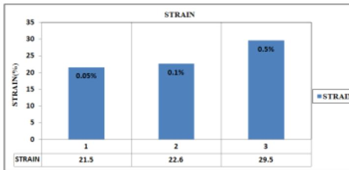
Fig 6: Typical Bar Graph Represents Strain Increasing Value of GFRP Modified With MWCNT-CNF
