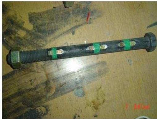
**Figure 2** Bolt Strain Gauge Arrangement Test Setup
