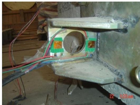
**Figure 3-a** Anchor Strain Gauge Arrangement Test Setup
