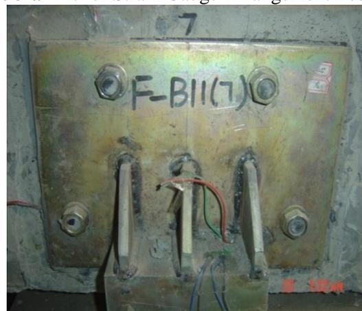
**Figure 3-b** Deviator Strain Gauge Arrangement Test Setup
