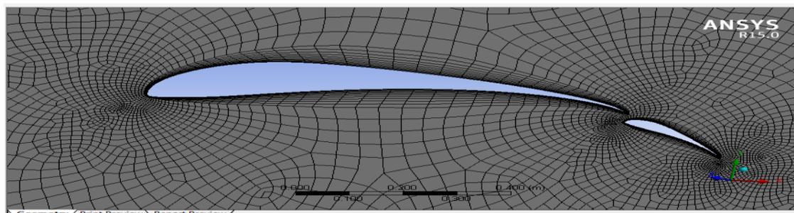
Fig 2 Airfoil S1223 With 1 Element
