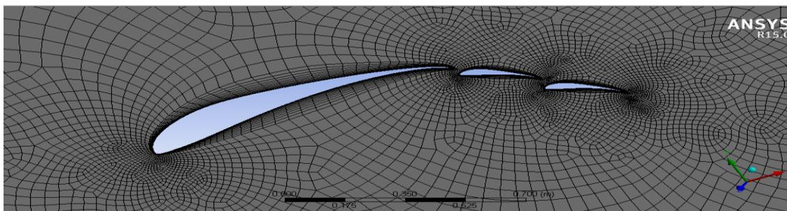
Fig 3 Airfoil S1223 With 2 Elements
