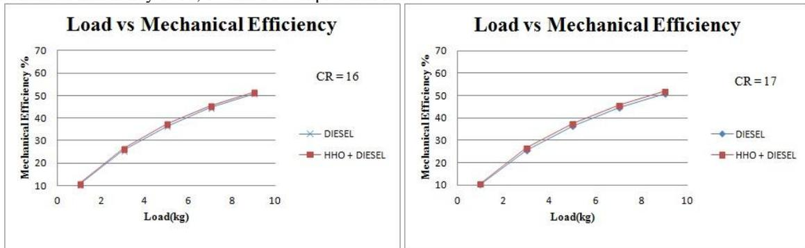
Fig. 12 Load Vs Mechanical Efficiency at CR 16 Fig. 13 Load Vs Mechanical Efficiency at CR 17
