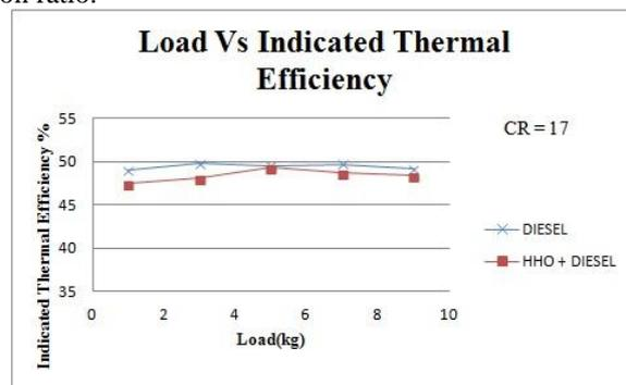
Fig. 7 Load Vs Indicated Thermal Efficiency at CR 17
