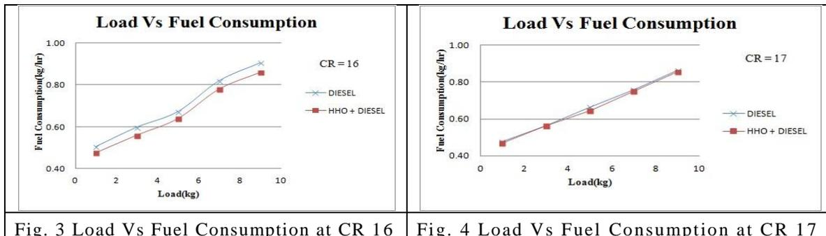
Fig. 3 Load Vs Fuel Consumption at CR 16
