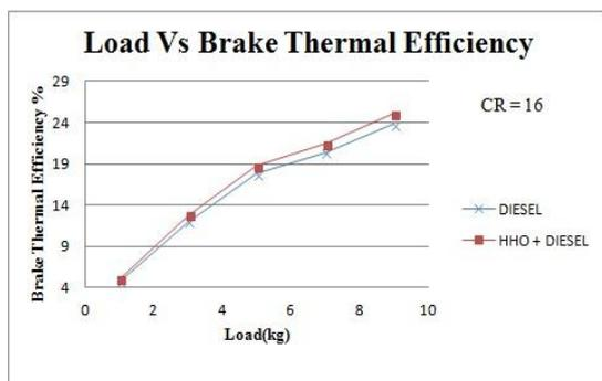
Fig. 9 Load Vs Brake Thermal Efficiency at CR 16
