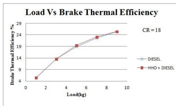
Fig. 11 Load Vs Brake Thermal Efficiency at CR 18
