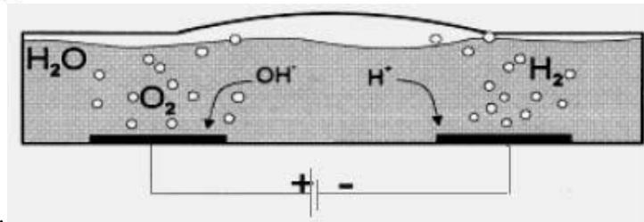
Figure 1 Schematic explanation of the process of electrolysis<sup>[2]</sup>
