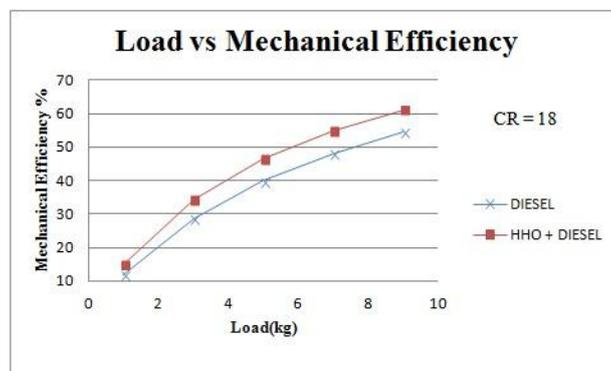
Fig. 14 Load Vs Mechanical Efficiency at CR 18
