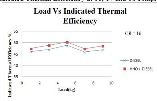
Fig. 6 Load Vs Indicated Thermal Efficiency at CR 16
