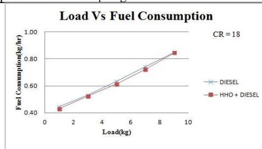
Fig. 5 Load Vs Fuel Consumption at CR 18
