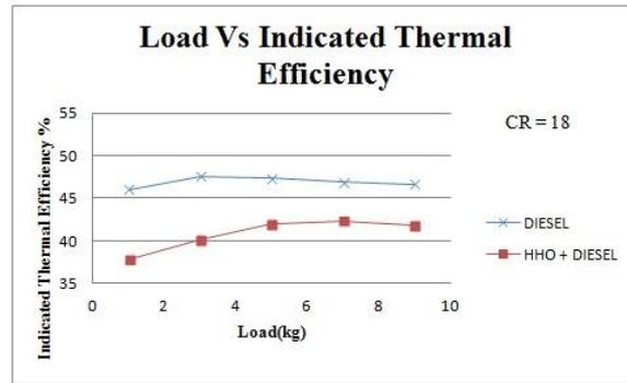
Fig. 8 Load Vs Indicated Thermal Efficiency at CR 18
