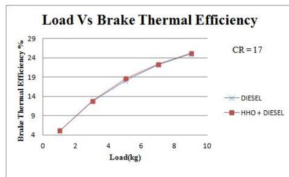
Fig. 10 Load Vs Brake Thermal Efficiency at CR 17
