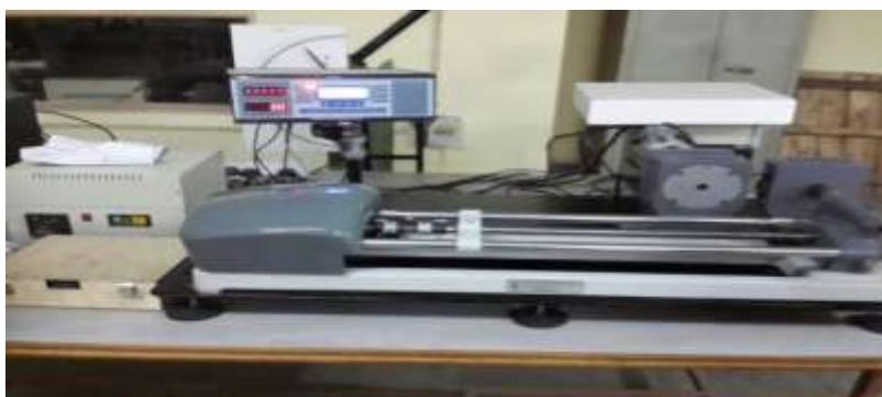
**Figure4.16** Extensometer tensile Testing Machine
