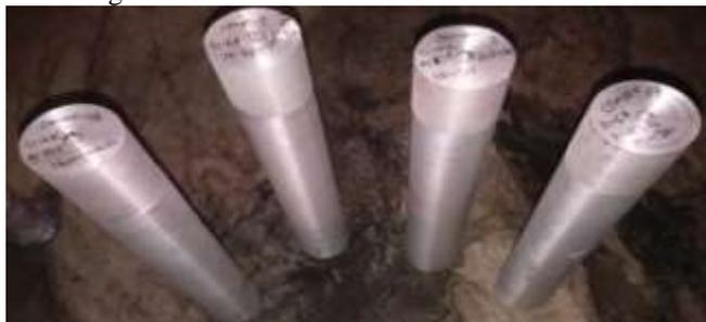
For the ultrasonic testing the whole machined sample was used, as this testing is also a Non-destructive testing so there is no harm to sample after the testing. Hence the samples were directly used for the ultrasonic testing. Ultrasonic Flaw Detector machine set up is used to detect the flaws if any present in castings produced.
