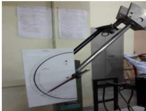
**Figure 4.21** Izod Impact Testing M/C
