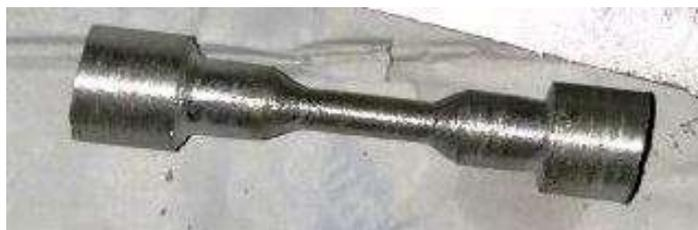
**Figure 4.15** Test Specimen of UTM
