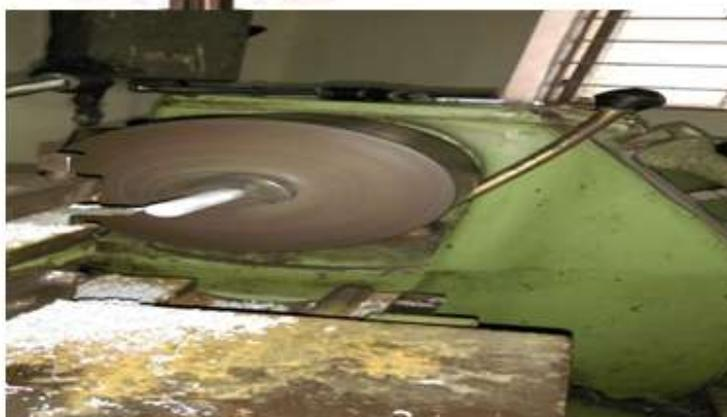
**Fig 3.13** machining of specimen for tensile test and specimen
