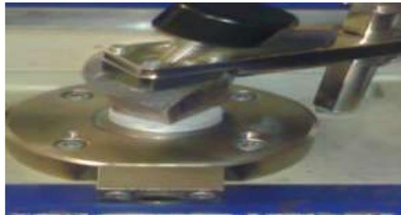
**Figure 4.8** Clamping Platform of Spectro Test Machine
