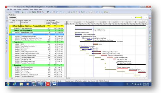
Fig-6 scheduling of a project by using Primavera
