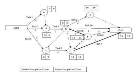
Fig-7 shows critical path method
