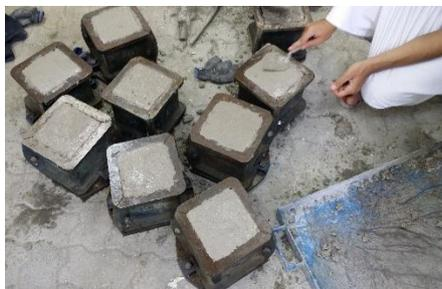
Fig.8 Casting of GPC Cubes
