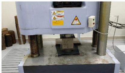
Fig.16 Testing of Cubes
