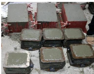
Fig.10 Casting of Solid Blocks
