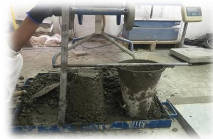
Fig.9 Slump Test for GPC
