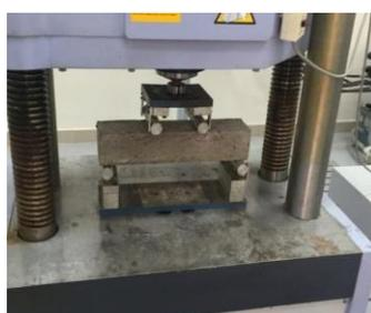
**Fig.18 Flexural Strength of Prism**
