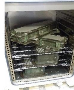
Fig.15 Prisms in Heat Chamber
