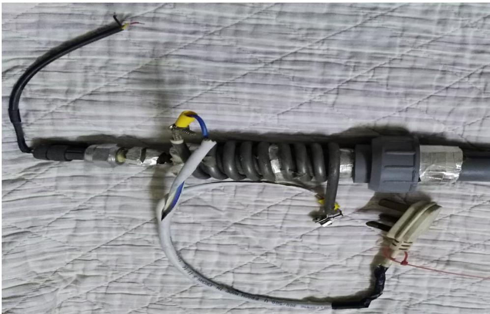
**Fig.2.** Electric resistance heater coil wrapped helically around outer diameter of evaporator section
