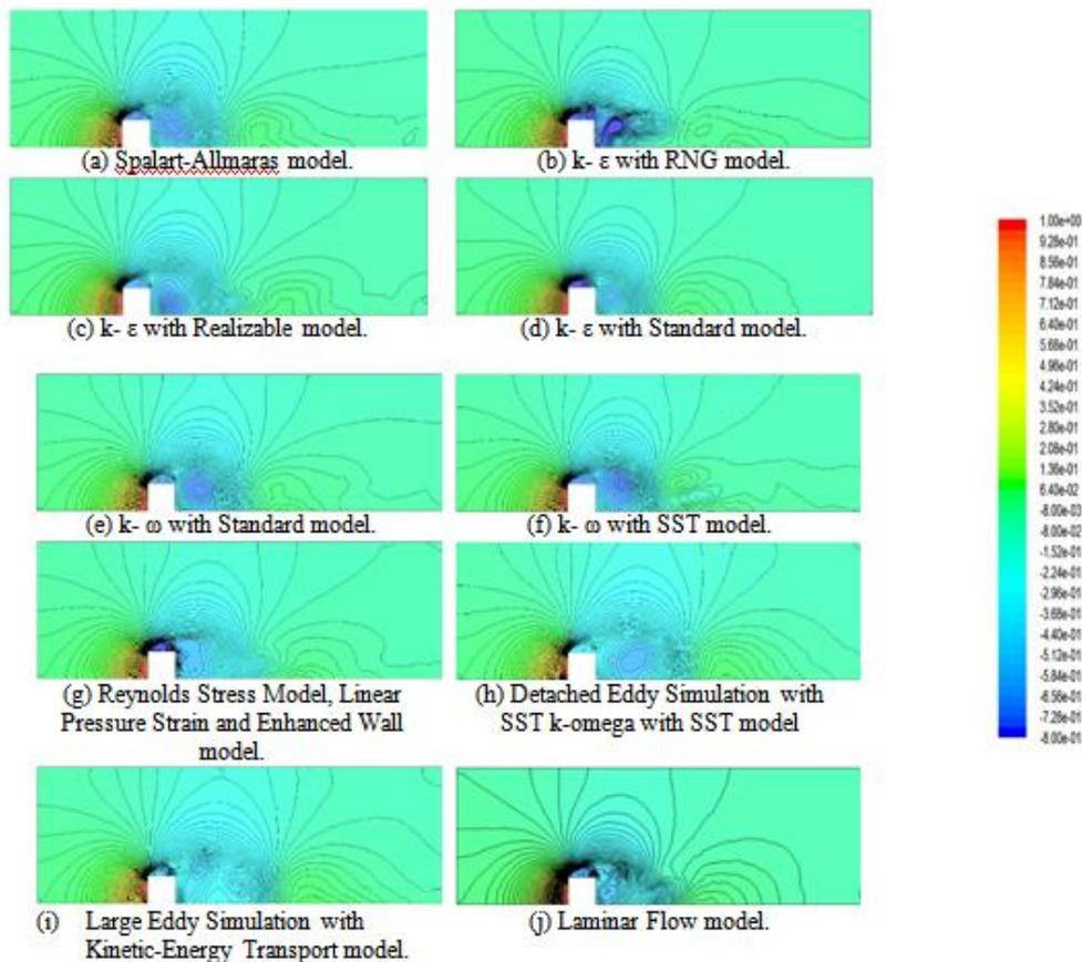
Fig. 3 Longitudinal cross sections at the middle of cube showing the contours of pressure coefficient
