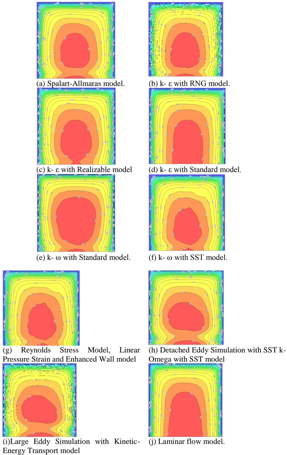
**Fig. 4** Distribution of the contours of pressure coefficients on windward face
