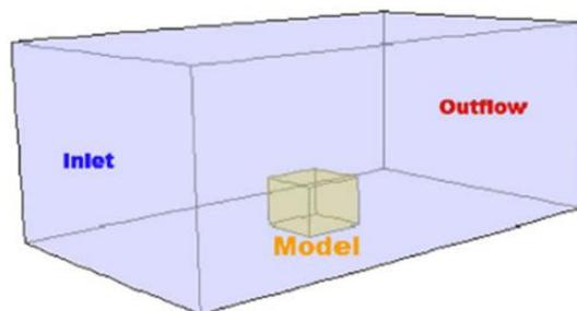
Fig.(1 –a) Schematic illustration of 3D Domain of Cubic building
