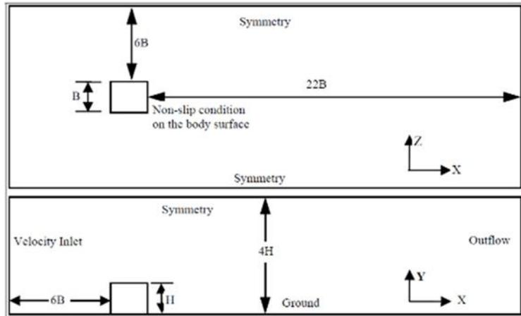
Fig.(1-b) Dimensional properties of 3D model of Cubic building
