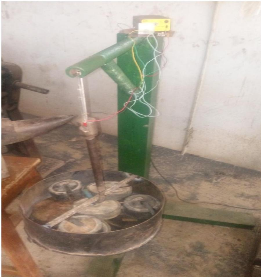
Plate 1: Developed Indigenous Strain Gauge
