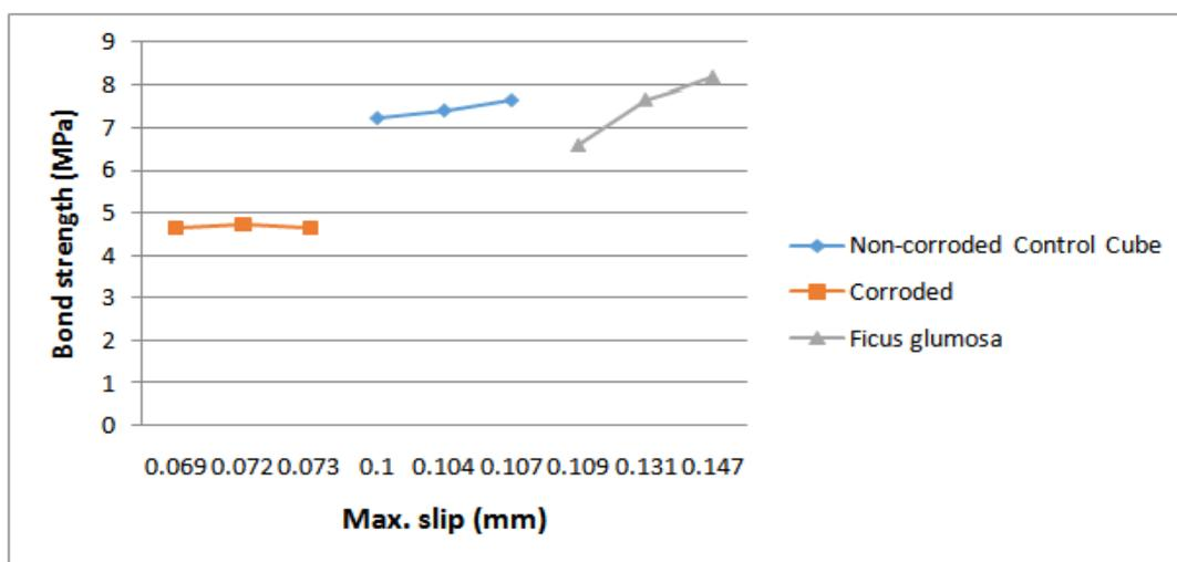
**Figure 3.4:** Average Results of Pull-out Bond Strength Test ( $\tau$ ) (MPa) (Bond Strength versus Maximum Slip)
