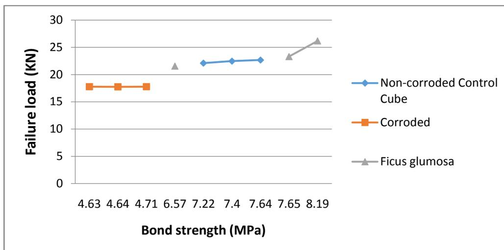
**Figure 3.3:** Average Results of Pull-out Bond Strength Test ( $\tau$ ) (MPa) (Failure loads versus Bond Strengths)
