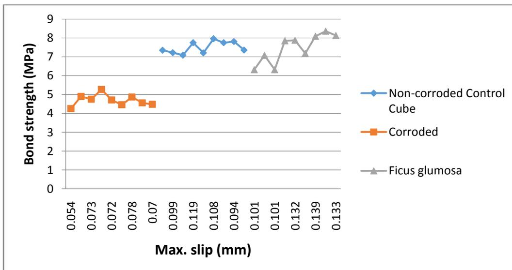
Figure 3.2: Summary Results of Pull-out Bond Strength Test ( $\tau_u$ ) (MPa) (Bond Strength versus Maximum Slip)
