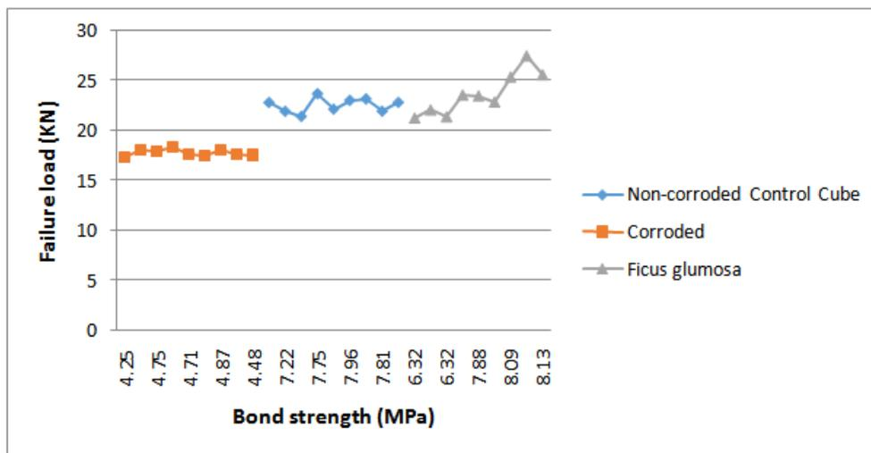
Figure 3.1: Summary Results of Pull-out Bond Strength Test ( $\tau_u$ ) (MPa) (Failure loads versus Bond Strengths)
