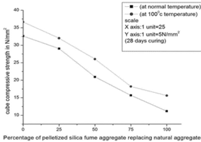
Fig 2. Superimposed Variation of cube Compressive strength vs SFA
