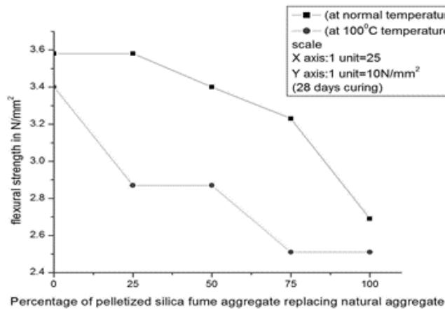
Fig 3. Superimposed Variation of flexural strength vsSFA
