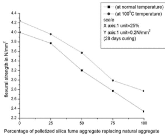
Fig 4. Superimposed Variation of flexural strength based on I.S.CodevsSFA
