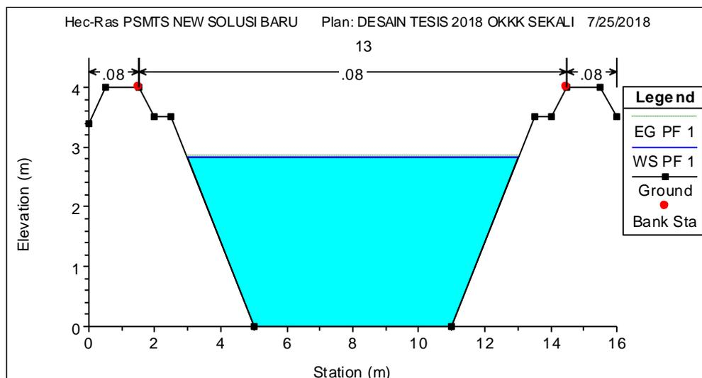
Figure 7. Cross Section Simulation P.1 SS.1-MH.1 (Source: Analysis)
