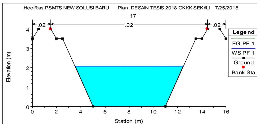
Figure 9. Cross Section Simulation P.18 SS.3-MH.3 (Source: Analysis)
